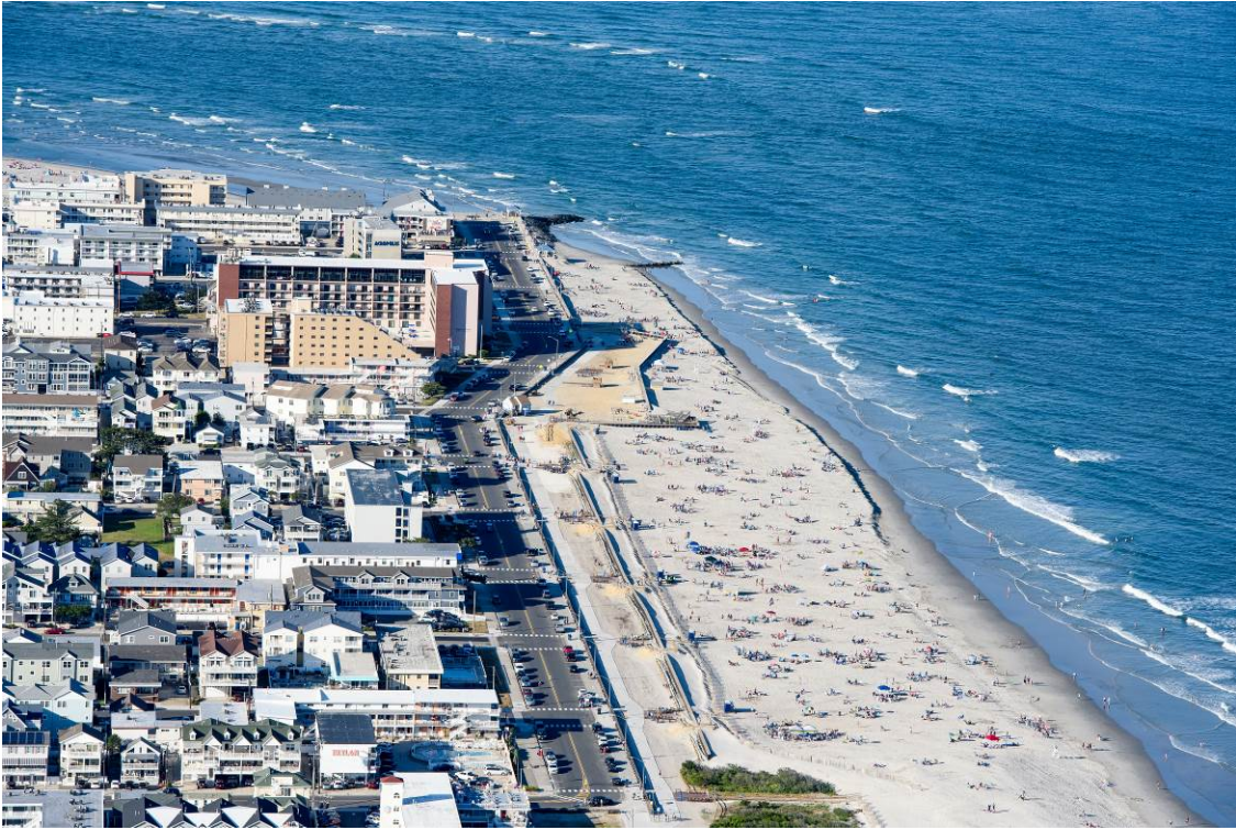
Figure 5. This view of the North Wildwood oceanfront beach extends from 13 th Avenue north to the 2 nd Ave. jetty. and shows the steel wall extended to 12 th Avenue and the sand added to the oceanfront shoreline derived from the City of Wildwood beaches. Photograph date is June 13, 2020 (photos by Ted Kingston). The scarp at the berm extends between 3 rd Avenue and 8 th Avenue on the beach.
