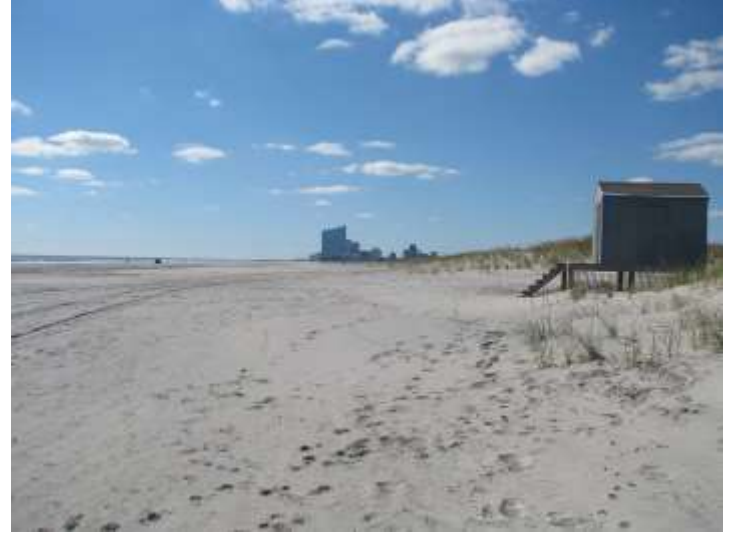
Figure 7b photo was taken looking south on October 15, 2015. The wide beach berm absorbed the full impact of the early October 2015 northeast storm event, first of a series in this El Nino season. There's no wrack line or indication wave run up reached anywhere near the seaward dune toe during the storm.
