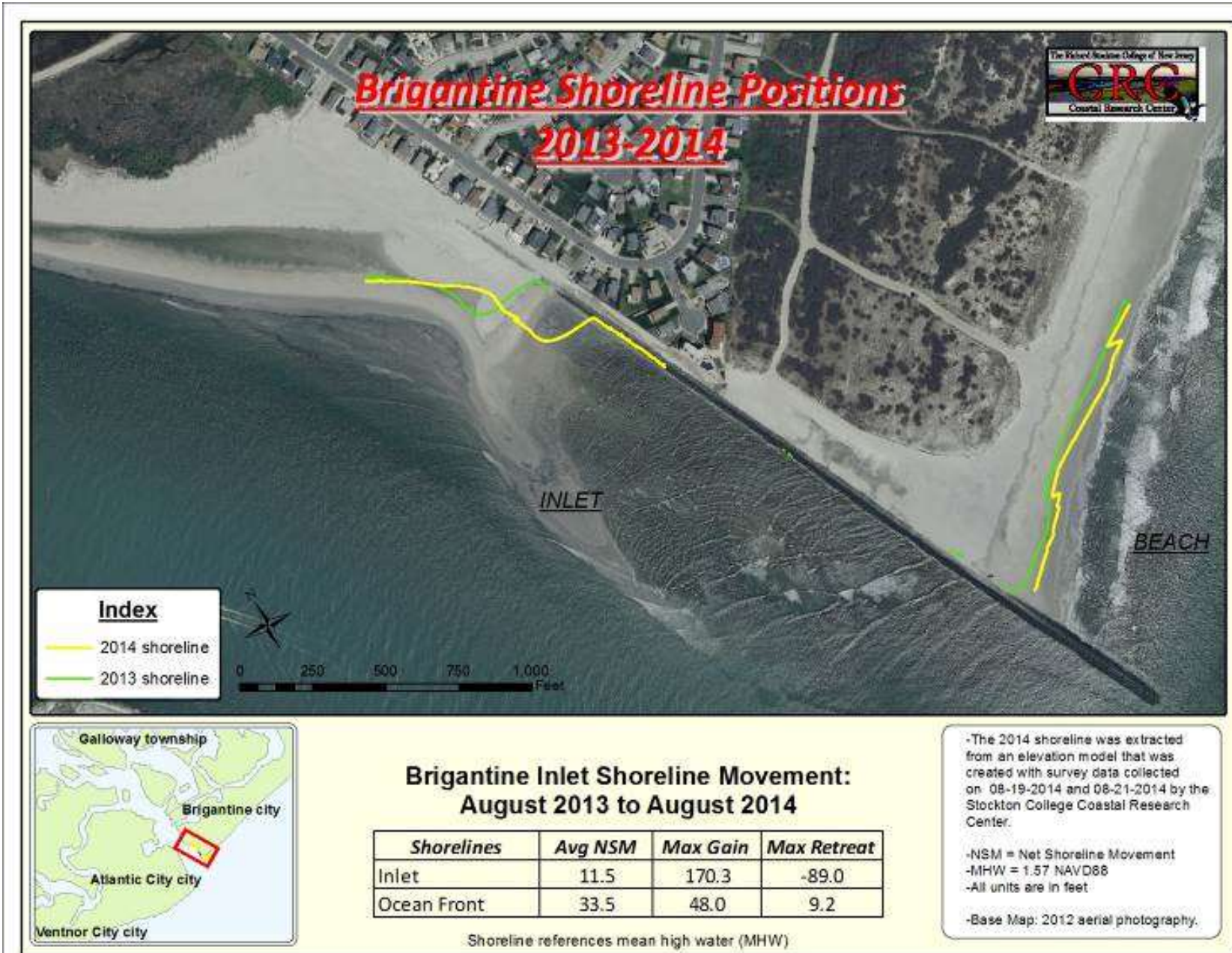
Figure 36 - Shoreline migration of Brigantine's beaches in the vicinity of Absecon Inlet where analyzed between 2013 and 2014. Shoreline positions are overlain on 2012 aerial photography. The average shoreline position advanced at both the inlet and ocean facing beaches over this study period.
