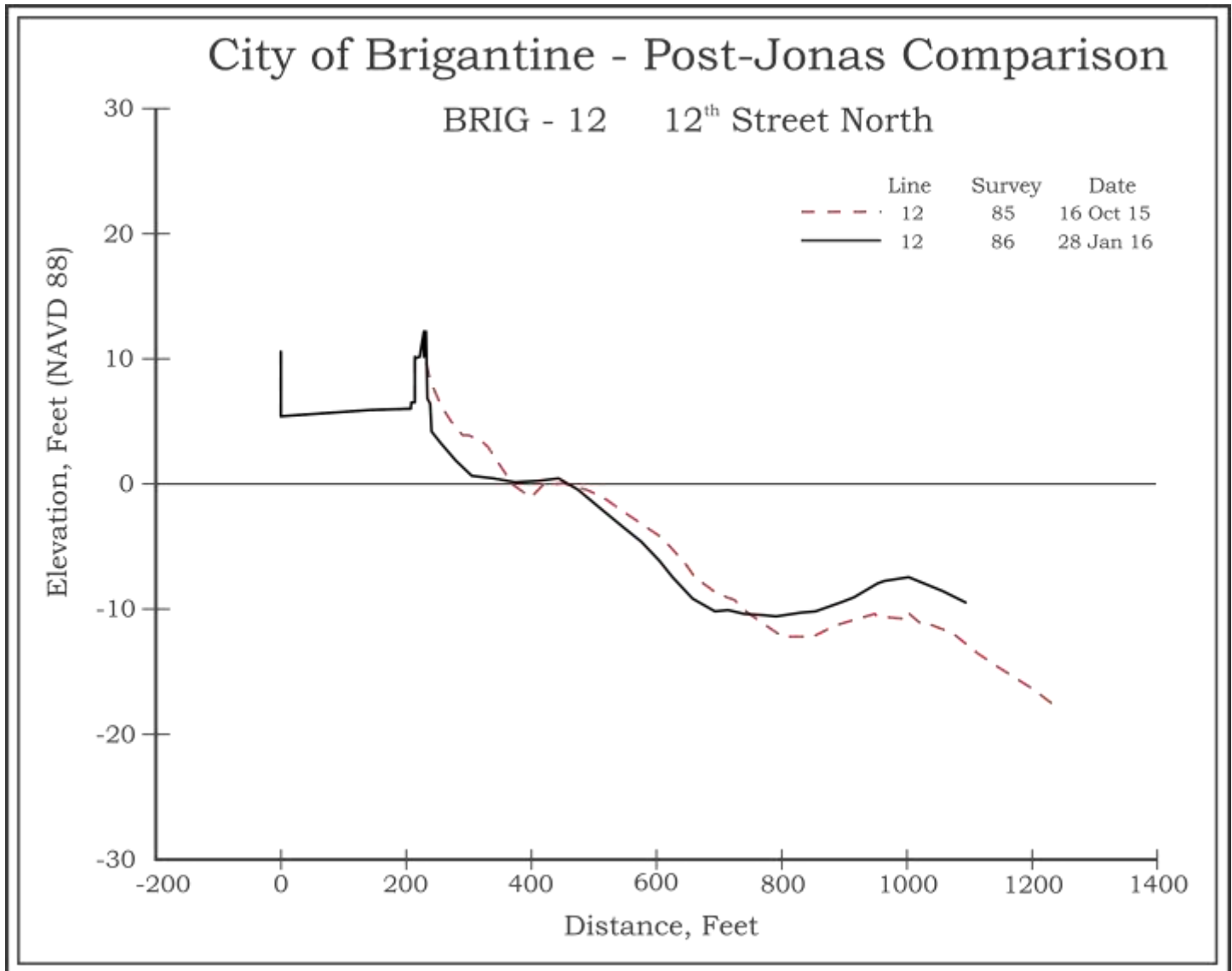
Figure 28 – Throughout 2015 this chronic erosional beach had rapidly lost sand and by the end of 2015 the sand volume had decreased by a massive 92.42 yds 3 /ft. of sand. This onshore and offshore sand loss diminished the beach width and elevation increasing the regions storm vulnerability. Jonas storm surge and waves removed the remaining beach berm cutting the beach landward to the revetment. Refracted wave energy during the storm scoured the remaining beach exposing the rocks along the promenade. Onshore the site lost another 12.22 yds 3 /ft. of sand. A storm wave also scoured the nearshore slope removing an additional 14.08 yds 3 /ft. of sand but unlike the beach to the north sand was transferred offshore at this location forming a shore parallel bar with. The offshore deposition of 28 yds 3 /ft. of sand offset the onshore and nearshore losses resulting in a minor net gain of 3.95 yds 3 /ft. of sand at this site despite these onshore and nearshore erosion. The minor net gain indicates a modest influx of sand was still moving south from the “feeder beach” to this region during Jonas. However, with both the “feeder beach” and chronic erosion regions now depleted of sand it is extremely likely that accelerated erosion along the promenade revetment will increase the erosion rate towards the south along the remaining engineered beach. Efforts to nourish this region should be made to reduce the impact to the downdrift beaches.
