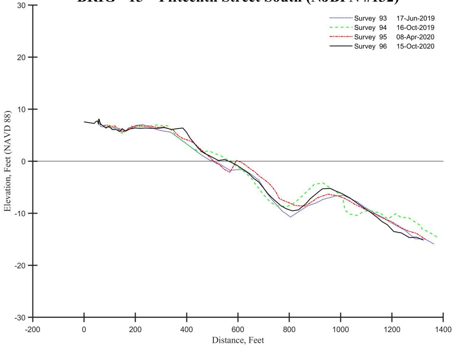
Figure 6c - At 15<sup>th</sup> Street South sand has been transported south to this location derived from the beach nourishment efforts further north since 1996. The offshore bar is extremely large for this location. 14.27 yds<sup>3</sup>/ft. in sand was deposited annually and the beach advanced 27 feet seaward between October 2019 and October 2020.
