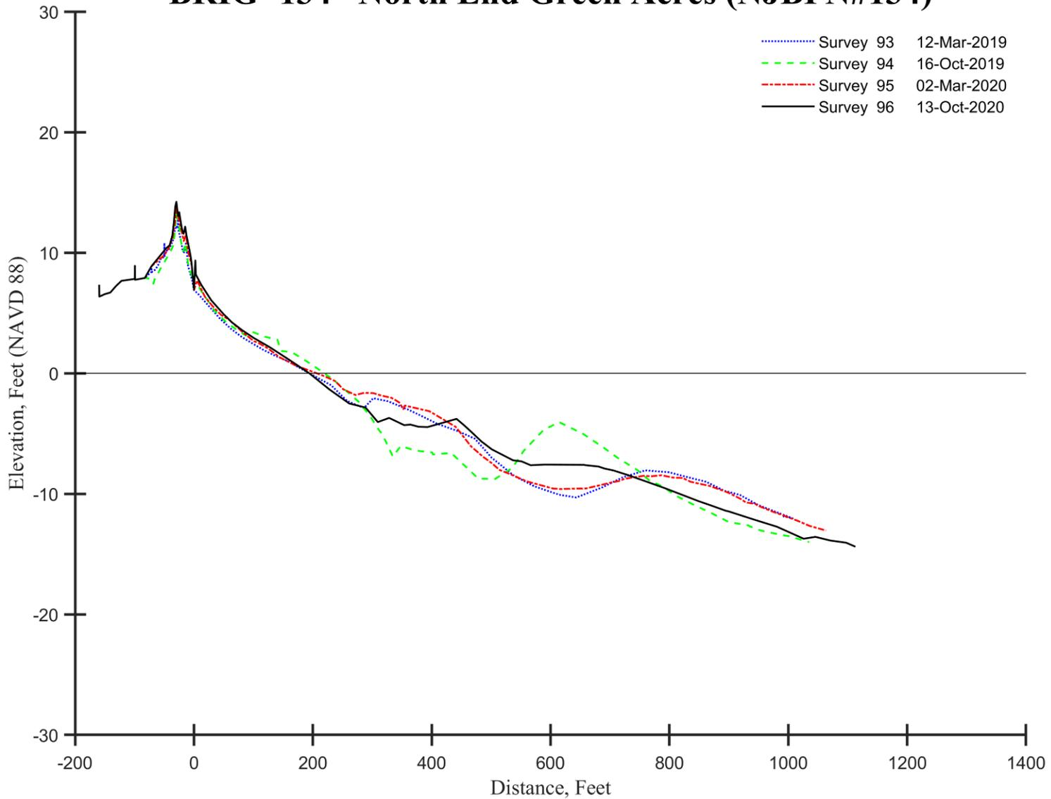
Figure 1c – The natural area beach has seen general sand accumulation on the dune and beach, while sand shifted dramatically offshore between a gentle slope into deeper water to a cross section with a deep trough seaward of the beach (Oct. 2019) and a very large offshore bar that generated 8.54 yds<sup>3</sup>/ft. in added sand. This bar flattened out with some sand shifting to the nearshore and on the beach.
