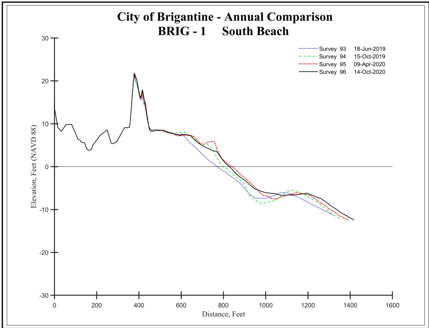
**Figure 9c – Positioned 600 feet north of the inlet jetty, this site has seen sand accumulate over the past 12 months perhaps because there have been few serious northeast storms to drive bar sand into Absecon Inlet. The beach and nearshore regions gained most of the 20.75 yds<sup>3</sup>/ft. allowing the shoreline to advance 29 feet seaward.**
