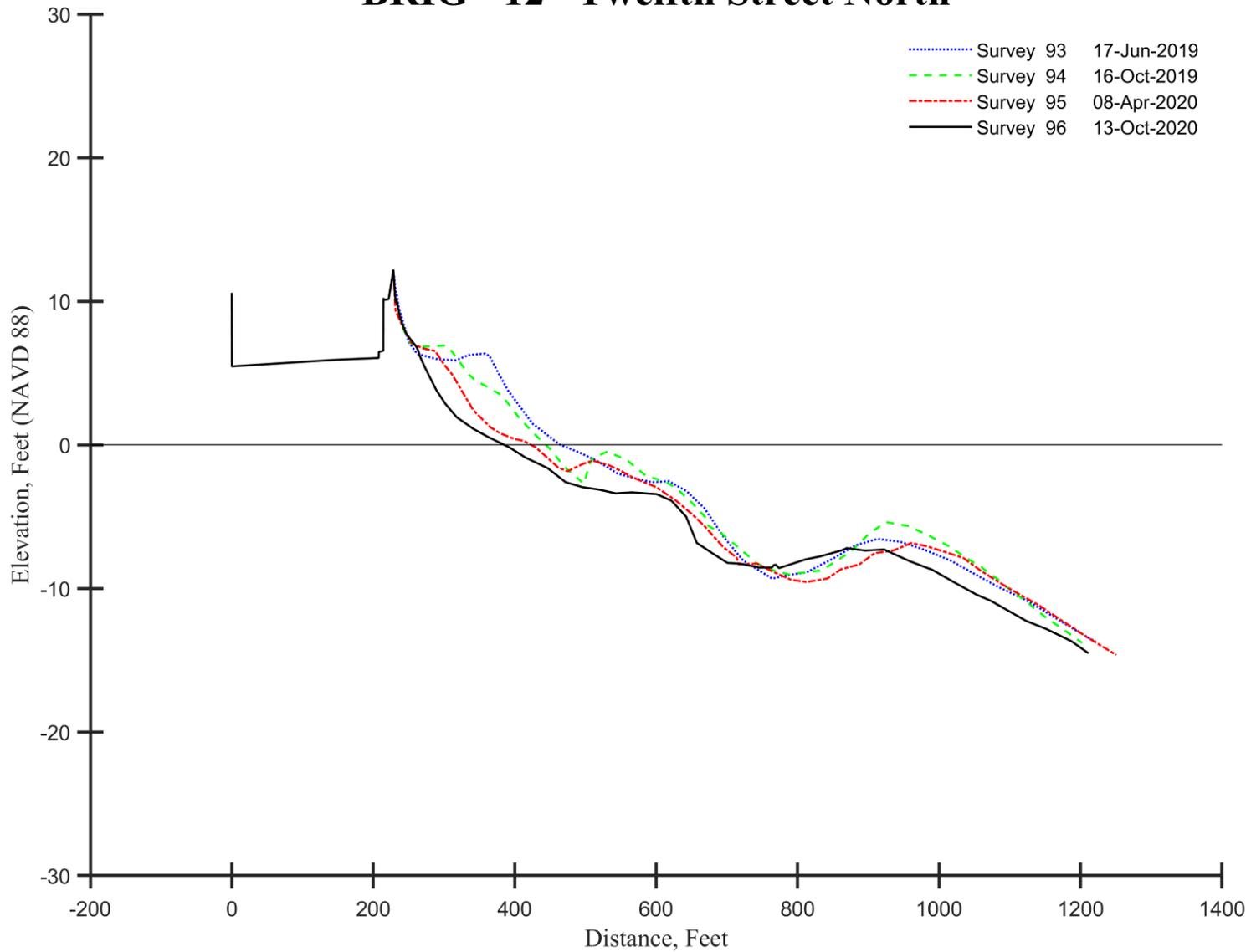
Figure 3c - This profile site was restored by the USACE project with 160.43 yds<sup>3</sup>/ft. The summer of 2018 saw general beachface retreat, which continued through 2020. The remaining dry beach is 25 to 35 feet wide reducing the shore protection considerably. The annual change of 2019-2020 saw -52.63 yds<sup>3</sup>/ft. with a 59-foot shoreline retreat by October 2020).
