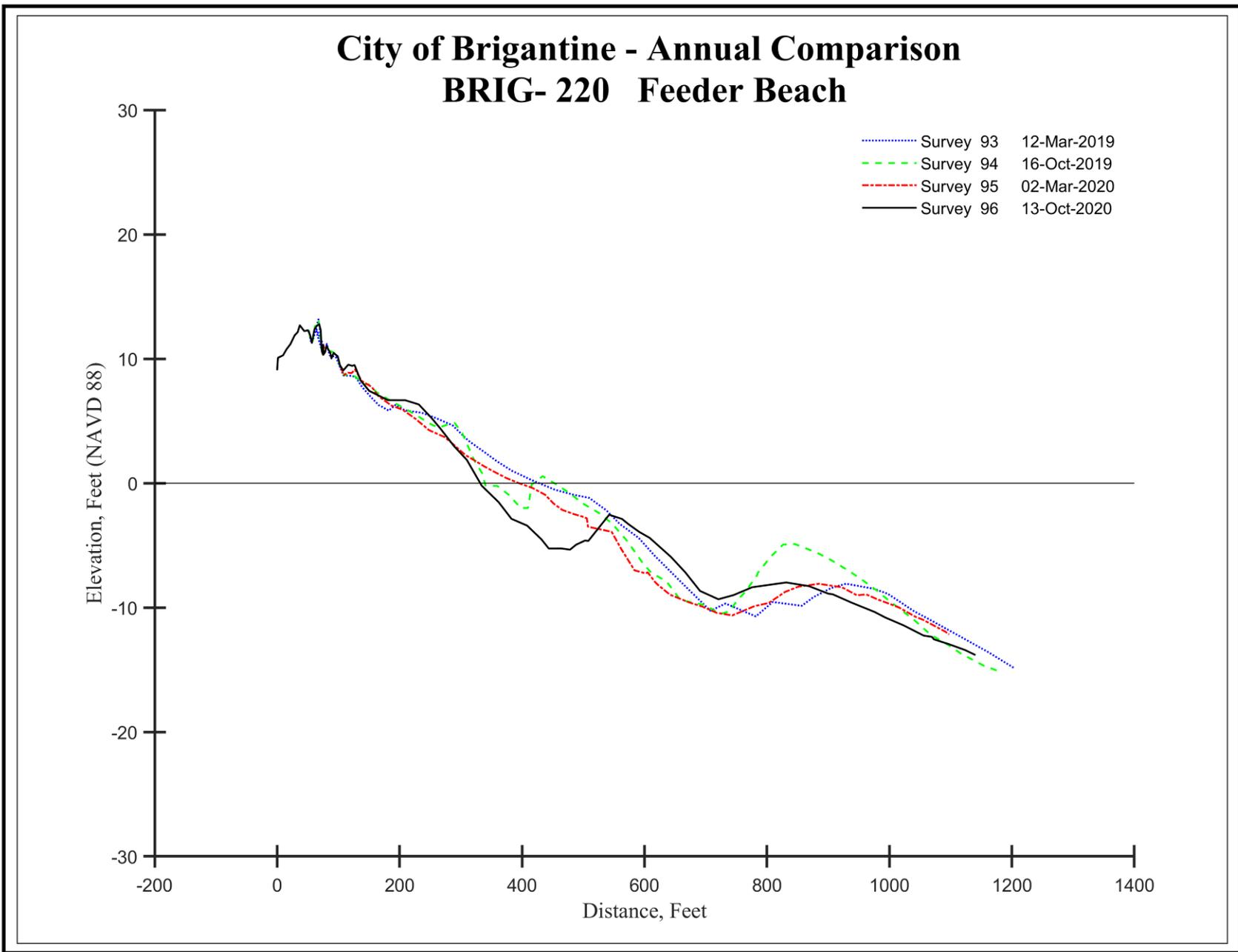
Figure 2c - Sand placed here by the USACE has remained stable between the dune and the beachface while extensive changes occurred offshore where the trough became deeper and a large bar and a nearshore ridge of sand appeared in the October 2019 survey. The net annual volume change was 30.07 yds<sup>3</sup>/ft. October 2019 to October 2020, and the shoreline retreated 121 feet landward.
