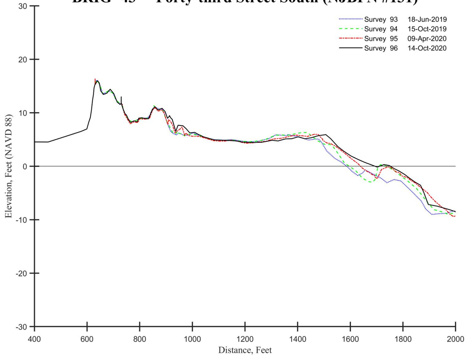
Figure 8c – This site continued to add sand to the beach, dunes and offshore areas. The annual sand volume increase was 24.06 yds<sup>3</sup>/ft. with a 16-foot shoreline advance. Sizeable sand volumes were added to the offshore bar system during the summer and into the fall of 2020.
