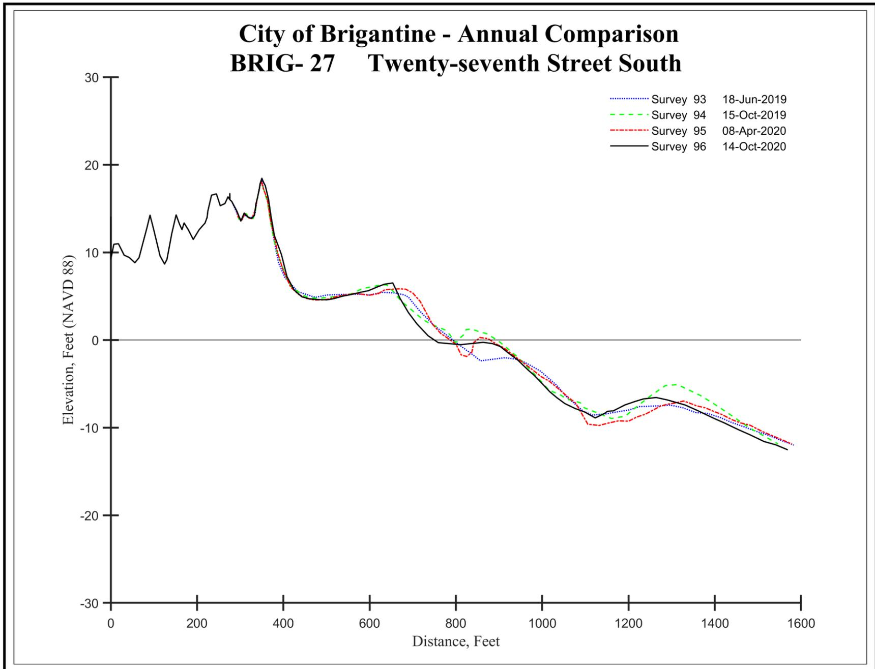
Figure 7c - 27<sup>th</sup> Street South survey saw beach retreat and sand volume losses this year for the first time in a long time, especially without significant storm activity. The site lost 22.55 yds<sup>3</sup>/ft. while the shoreline point retreated 145 feet.
