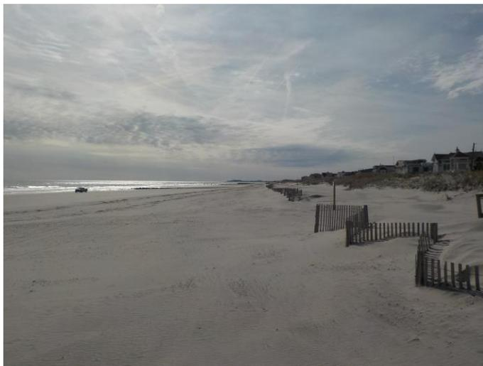
**Photoplate 4c – Photo taken November 8, 2018 showing sand extensively filling the 4-foot high snow fencing in one year. The beach width was sufficient to provide the supply.**
