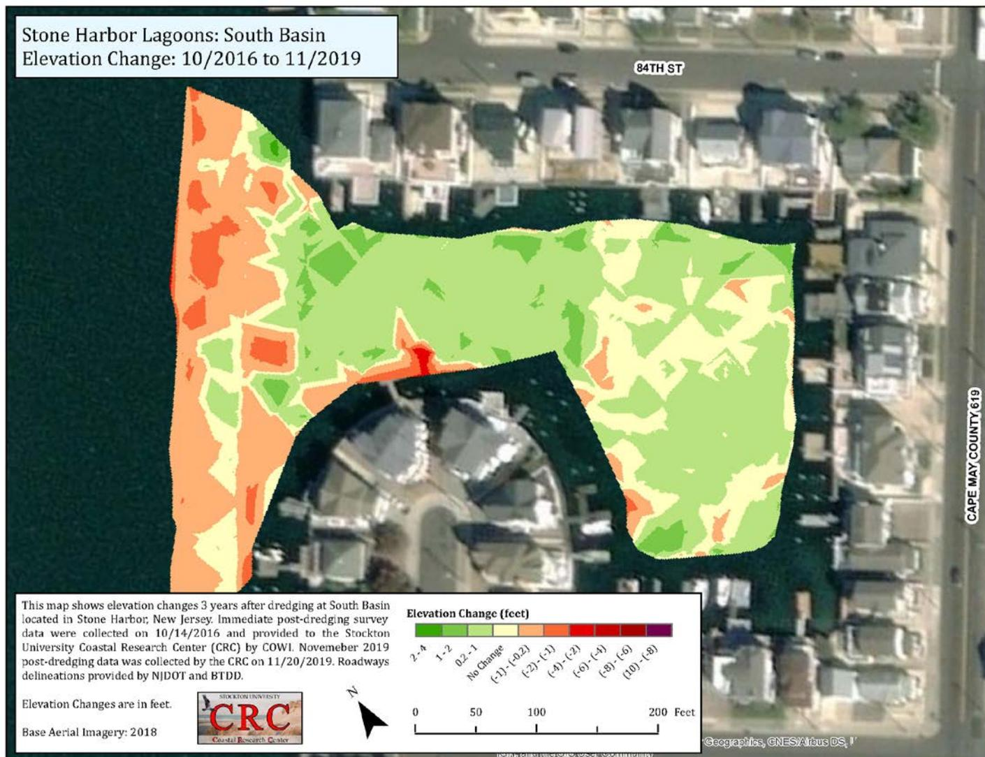
**Figure 9b. South Basin has performed in similar fashion to the post-dredging changes seen in the North Basin. Between 0.2 and 1.0 feet of sedimentation since dredging has appeared over three years across the main channel and to a lesser degree, within the inner basin, while entry point erosion has created deeper water where the Great Thorofare main channel joins the navigation channel into South Basin.**
