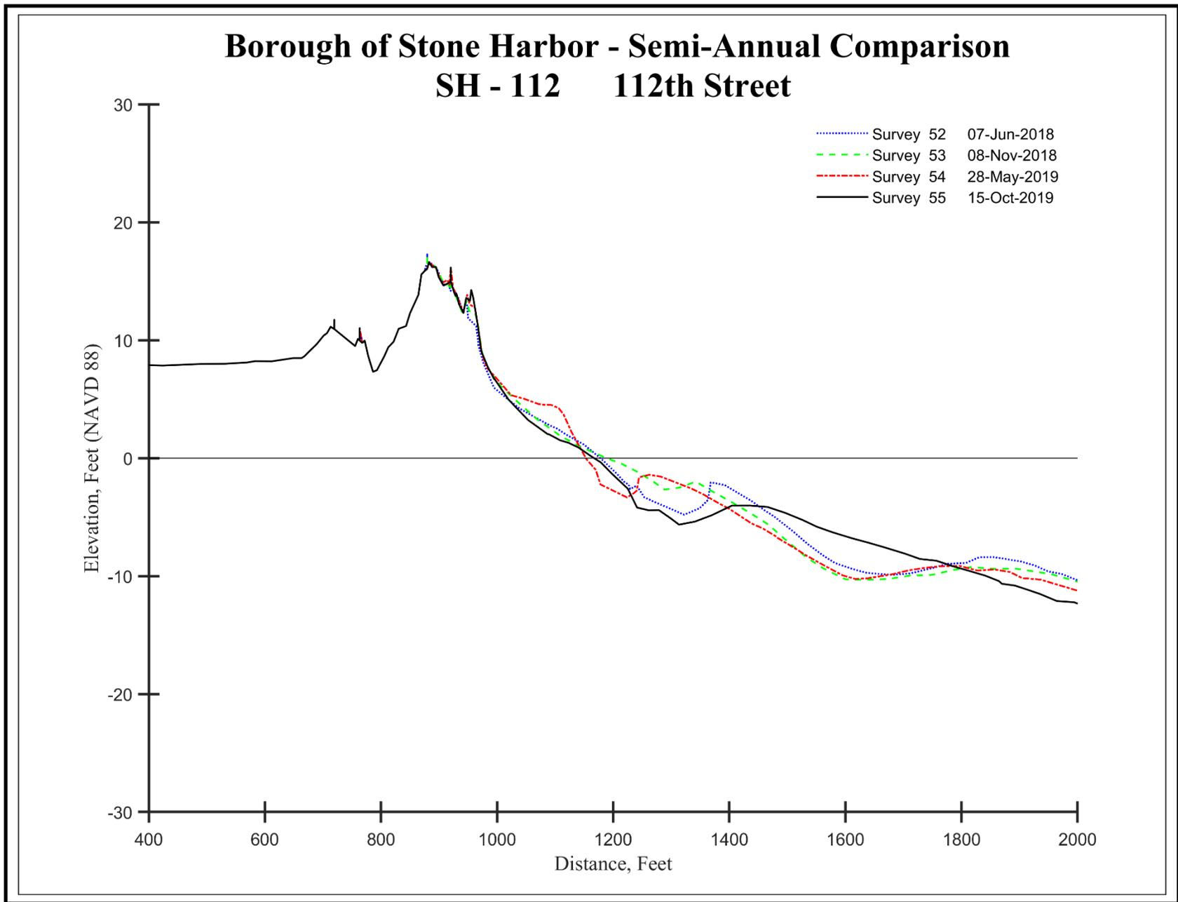
Figure 6d. The profiles at 112<sup>th</sup> Street lost the most sand over the past 18 months (-15.25 yds<sup>3</sup>/ft. and the shoreline retreated 11 feet). The May to October 2019 time interval produced a small decline in sand volume (-2.61 yds<sup>3</sup>/ft. with a 14-foot shoreline advance).
