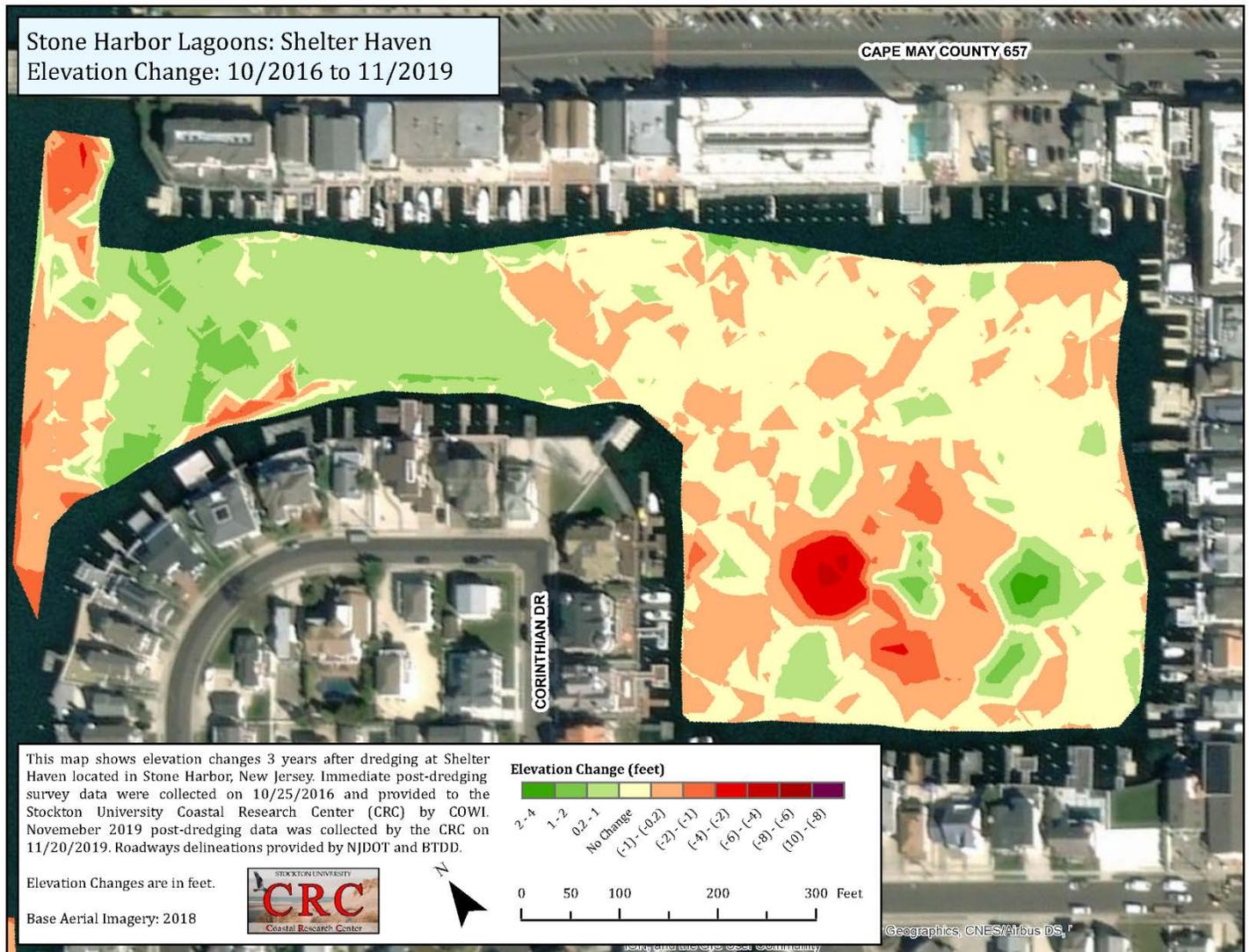
**Figure 11.** Shelter Haven is located just south of 96<sup>th</sup> Street and is similar in the pattern to the north where the inner basin is unchanged or marginally deeper, the entrance channel is up to a foot shallower and the entry point from Great Thorofare has seen sediment erosion at the point where the eastern Great Thorofare channel margin is met.
