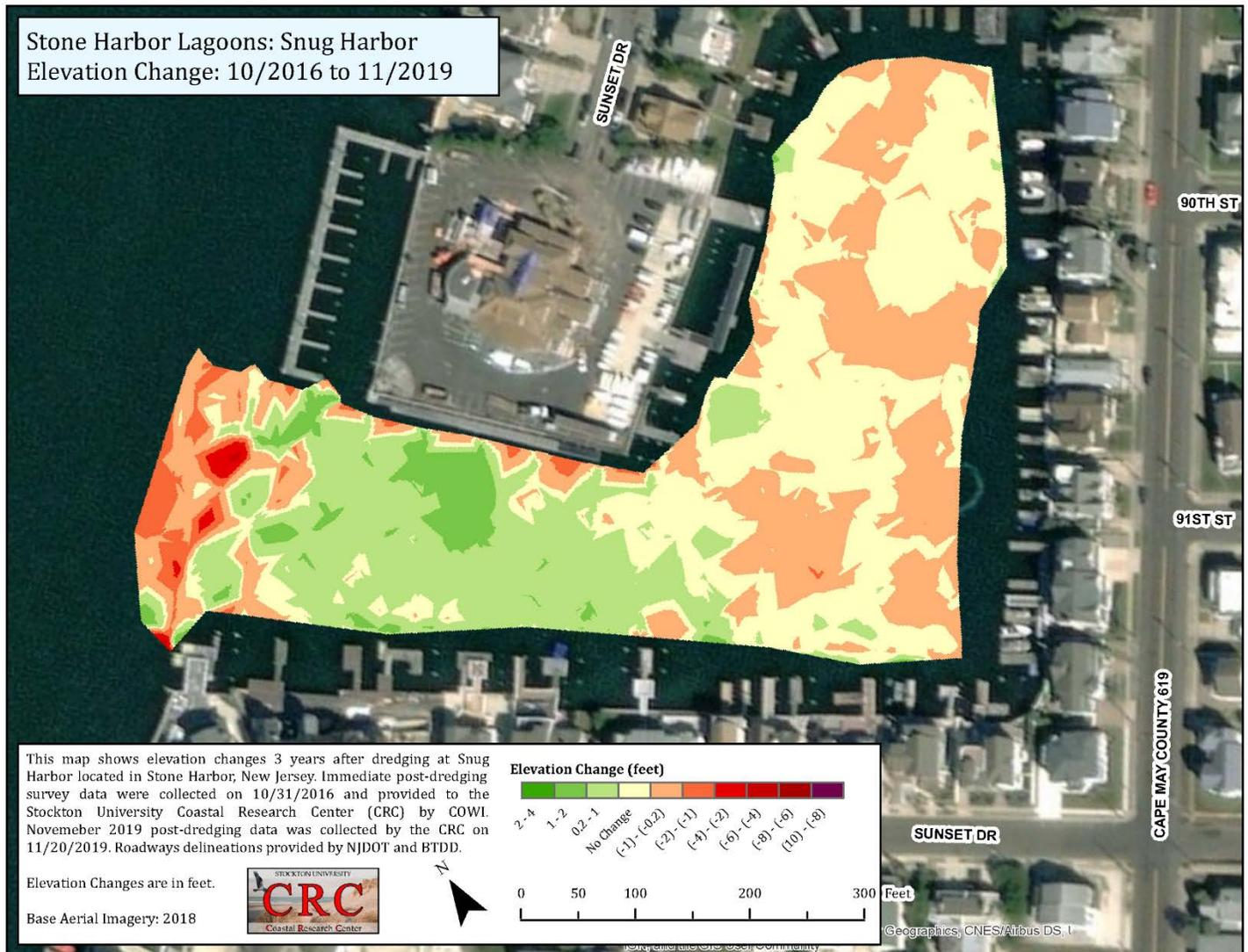
**Figure 10. Snug Harbor shows between zero and 1.0 feet of deepening in the inner basin, while showing 0.2 to 2.0 feet of shallower areas within the entrance channel. A complex set of bands across the entrance show areas of deeper depths with patches of shallower areas. These range from -3.0 to zero to 1.0 foot shallower. The survey covered a zone into the main channel at the yacht club.**
