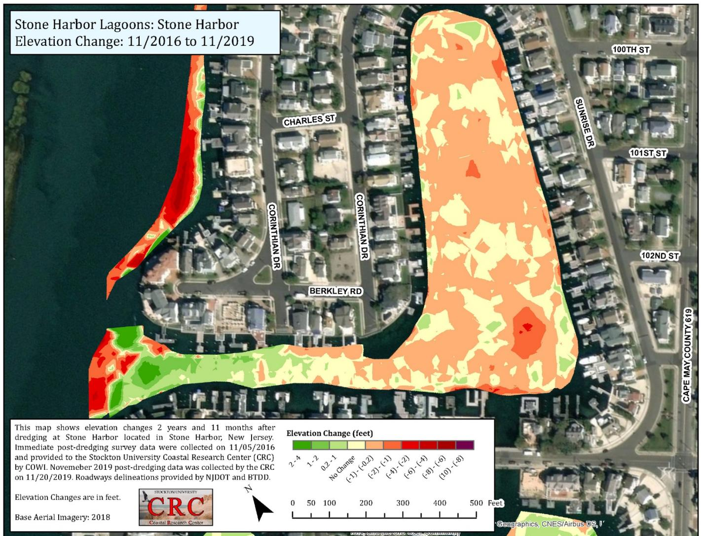
**Figure 12. Stone Harbor Lagoon displays a consistent pattern associated with the northern basins where the inner basin has remained as dredged or become marginally deeper (-0.2 to -1.0 feet) while the entrance channel has become shallower since November 2016. Sediment erosion has impacted the entry point with up to 4 feet of lost material at the southern margin bulkhead. This erosion extends north of the entrance as well, reaching 10-foot greater water depths.**
