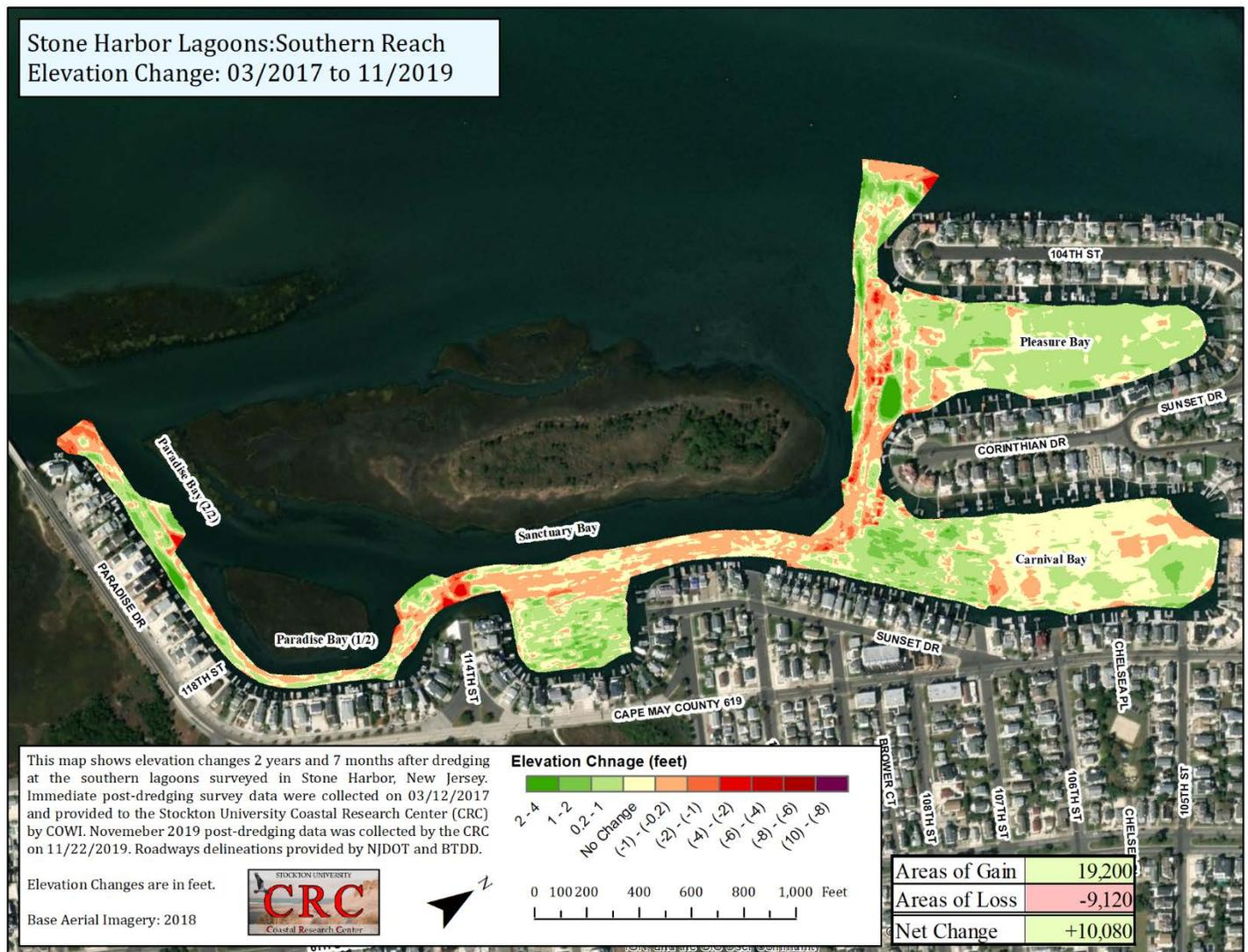
**Figure 16.** This map ties together five separate locations above into a composite for Sanctuary Bay and its associated lagoon basins. The entire region gained just over 10,000 cubic yards of sediment since dredging was completed. This was dominated by sediment deposition in Pleasure and Carnival Bays. The access route among the four developed lagoons appears to be getting deeper since dredging with minor exceptions along Paradise Bay channel.
