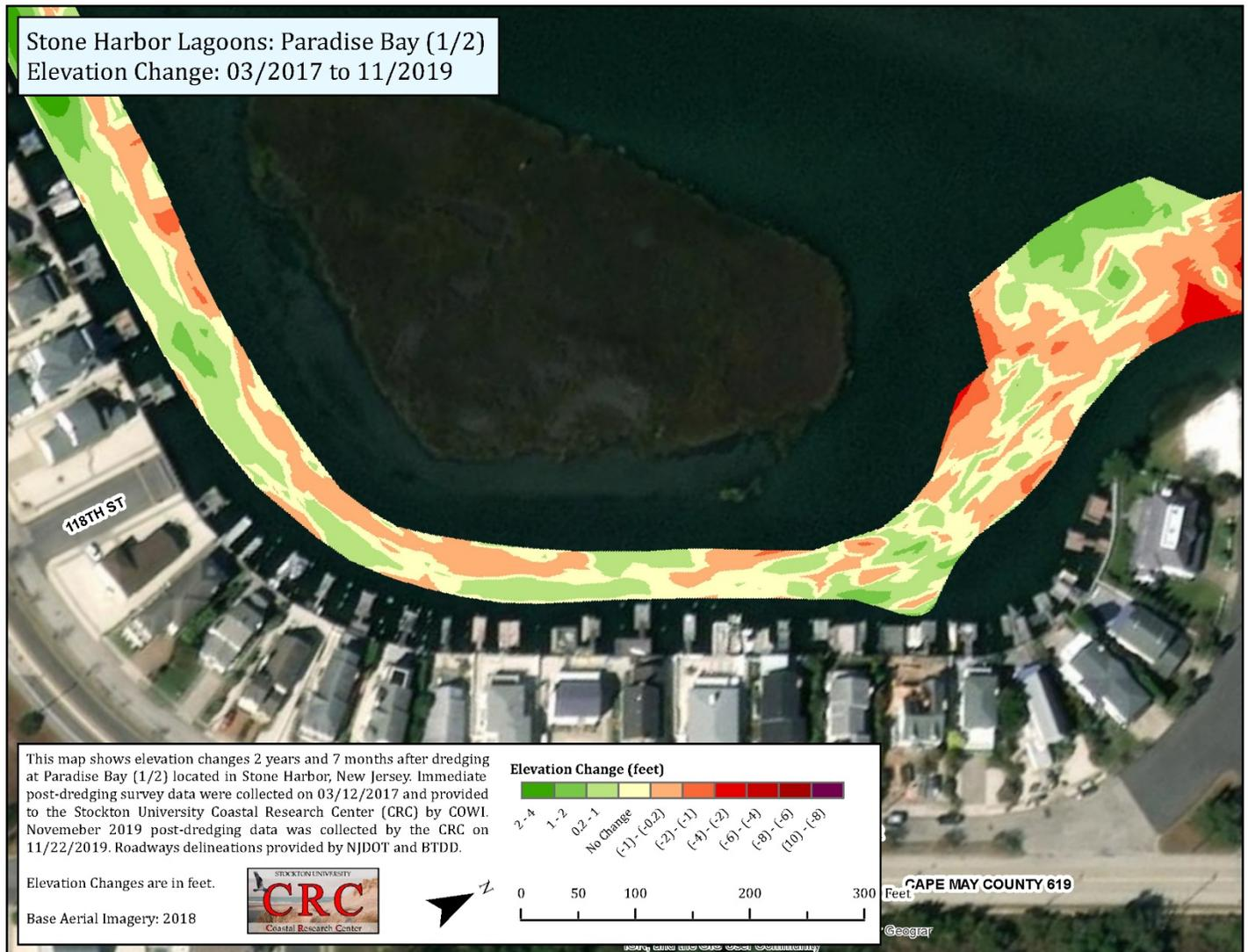
**Figure 15a.** The northern end of Paradise Bay is a dug channel between development and a marsh bay island to the west. There is spotty pattern of accumulation, no change and erosion since March 2017 when dredging was completed. The pathway south between marsh islands west of this channel is shallower to the point of avoidance by larger vessels particularly at low tide.
