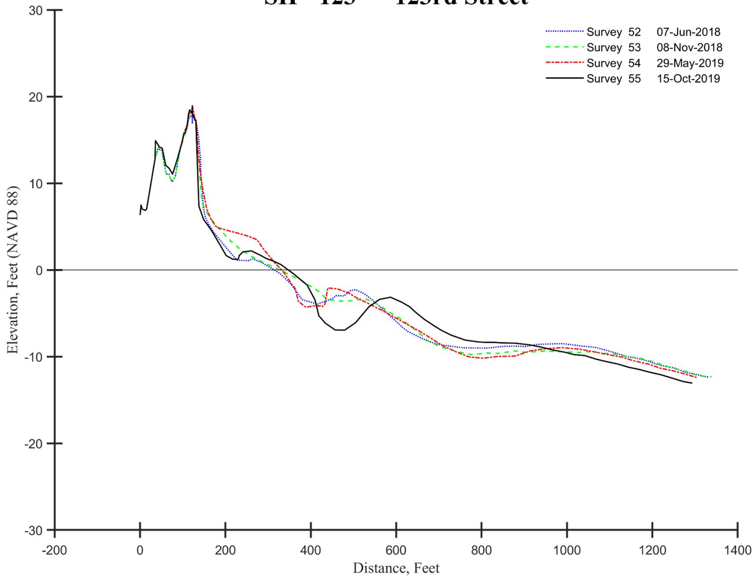
Figure 8d. 123<sup>rd</sup> Street saw nearshore bar accretion producing a decent beach berm by May 2019. Early storm events removed it and cut into the dune toe. The site lost 5.60 yds<sup>3</sup>/ft. over the past 18 months, but the shoreline advanced 15 feet seaward because of the October bar attachment. Offshore, a larger bar system appeared as well.
