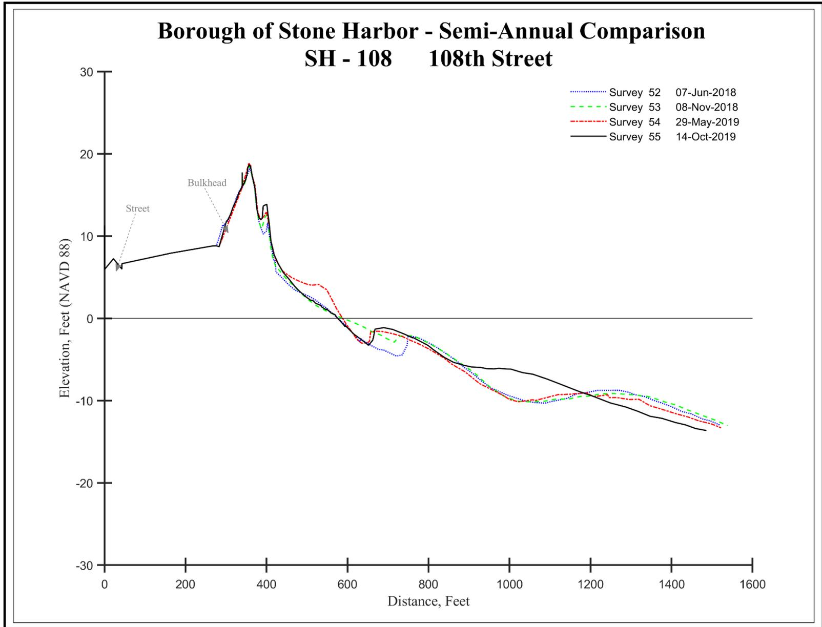
**Figure 5d.** The cross sections show dune development at the seaward fencing creating a new foredune. The May 2019 berm was quite pronounced along with multiple occasions where nearshore bars attached to the beach. Sand filled a trough offshore without generating a pronounced bar system here. The site gained 15.96 yds<sup>3</sup>/ft. with no change in the shoreline position over 18 months.
