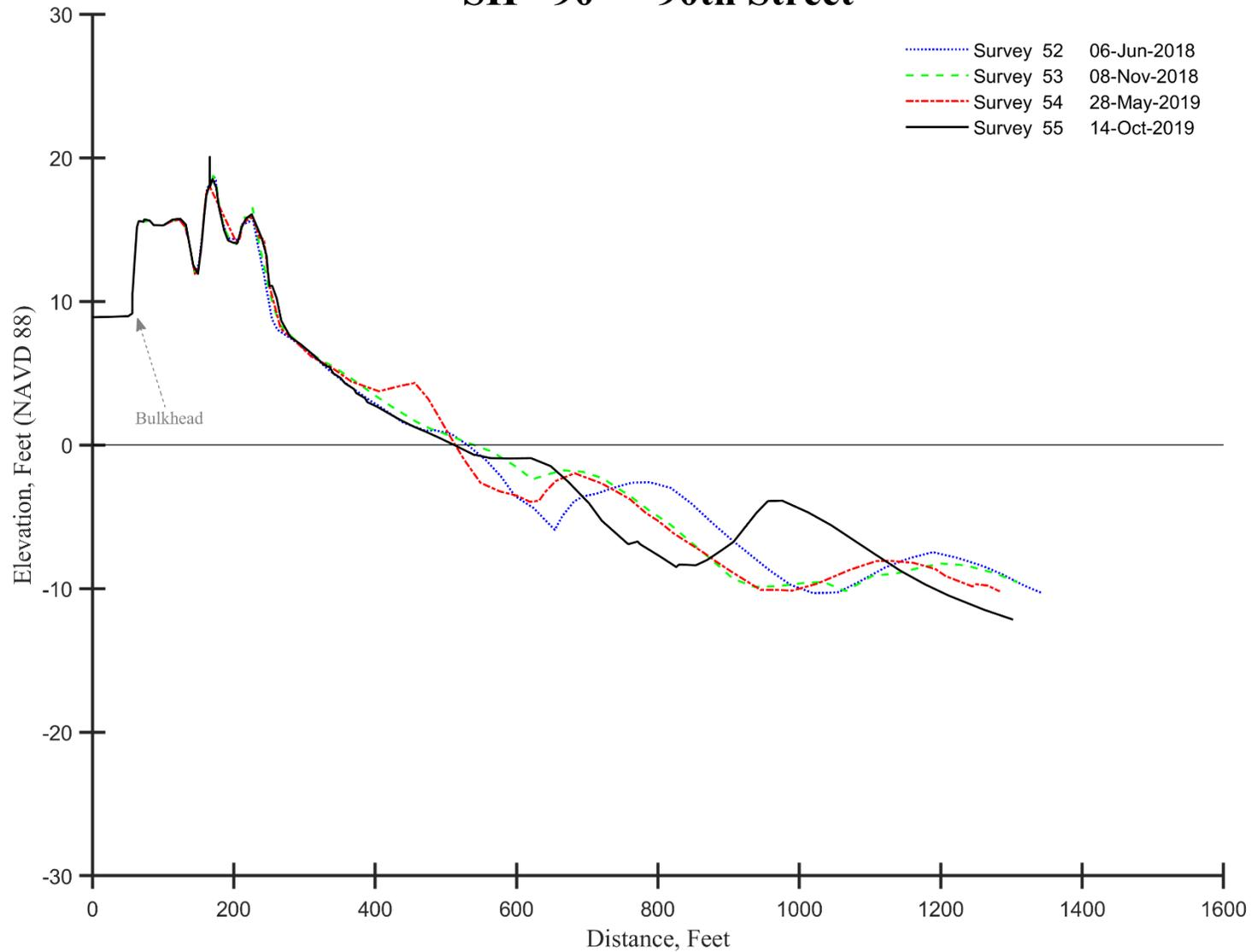
Figure 2d. The cross sections show minor additions to the dune and the May 2019 berm development. The beach slope returned to previous slopes by October 2019, while a very large offshore bar appeared at the 1,000-foot distance. The 18-month sand volume gain was 2.09 yds<sup>3</sup>/ft. (11.32 yds<sup>3</sup>/ft. May to October 2018) and the shoreline retreated 19 feet.
