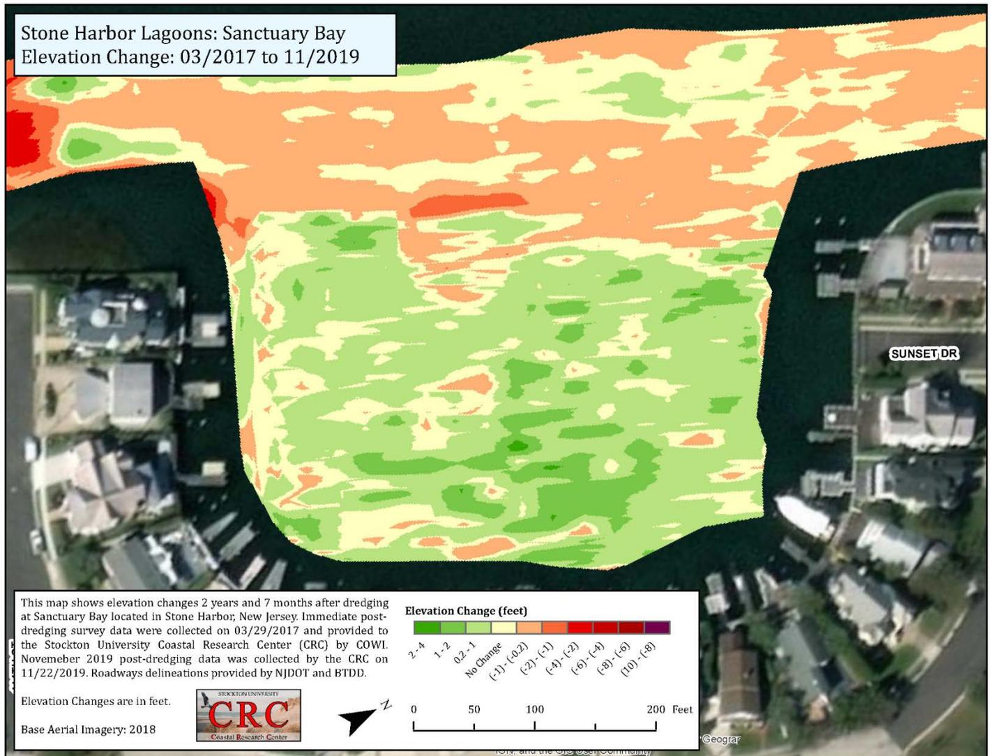
**Figure 14.** Sanctuary Bay lies east of the channel running south from the entrance to Carnival Bay and that exits at the bridge to North Wildwood. The excavated basin appears shallower by 0.2 to 2.0 feet in some spots, while the channel area is deeper by the same measure (0.2 to 2.0 feet). Substantial areas of no change still exist.
