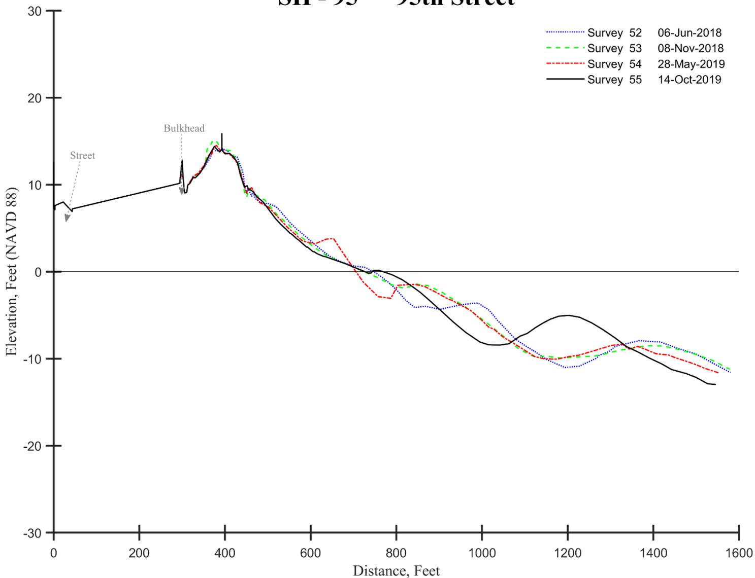
Figure 3d. The dunes and upper beach area saw little change in the past 18 months, but the same berm growth by May 2019 followed by its removal by October 2019 and the appearance of a very large offshore bar at the 1,200-foot distance required attention as to its cause. The site lost 0.44 yds<sup>3</sup>/ft. since May 2018 accompanied by a 23-foot shoreline advance.
