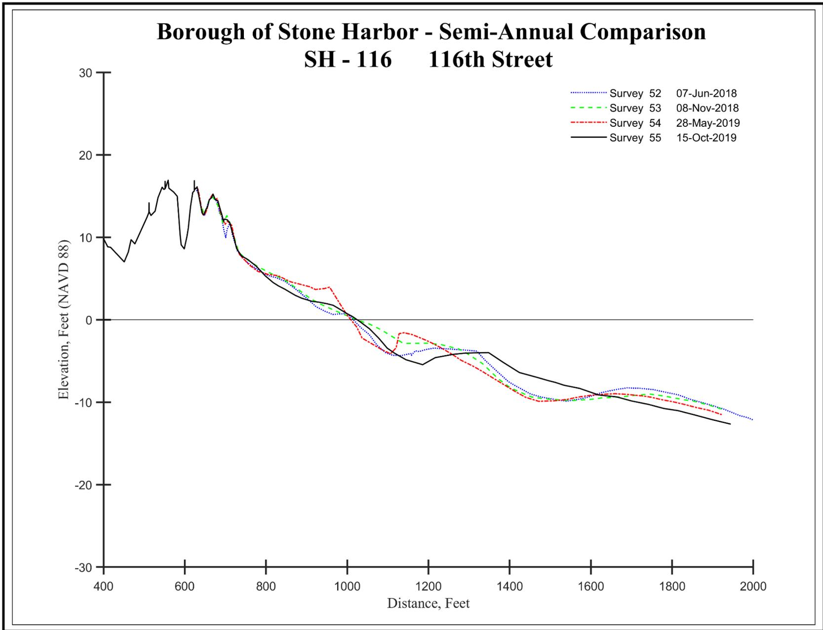
Figure 7d. The 116<sup>th</sup> Street location includes a double dune system which appears to have developed a new foredune peak adding to the dune volume. The beach produced a berm by May 2019 which was derived from the attachment of nearshore bars during the summer. This site lost 3.17 yds<sup>3</sup>/ft. over the past 18 months as the shoreline advanced 10 feet seaward.
