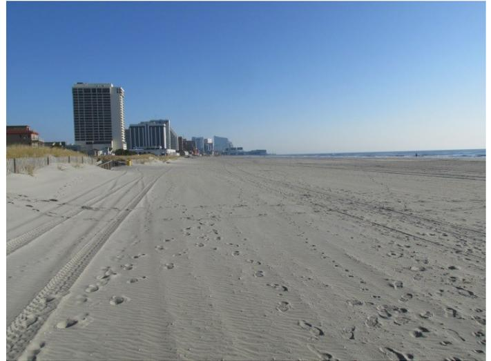
This site lies in the middle of the Federal shore protection project on Absecon Island where erosional loss has been minimal. On the left (December 1, 2014) one is looking north along the dune fencing placed relatively recently. The photo on the right was taken December 10, 2015 and shows that sand accumulated at the fence to half its original 4-foot height.
