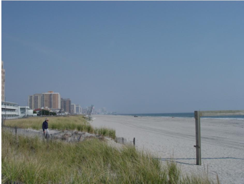
Figure 220. Dune growth by October 17, 2007 is very evident, with a slightly narrower beach as some sand moved south. The reduction amounted to about 15% of the original project width.
