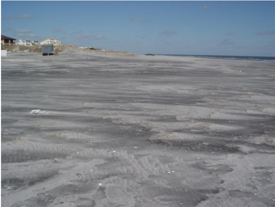
Figure 200. This beach is a beneficiary from sand migration south from the three episodes of beach nourishment at the northern end of the municipal development. The evidence appears as increased sand volume on the beach within 3 months of the project completion. The width of the dry beach today provides more protection for the old Brigantine Hotel, now the timeshares condominium, because this building has no dune in front of the bulkhead right at the seaward-facing building façade.
