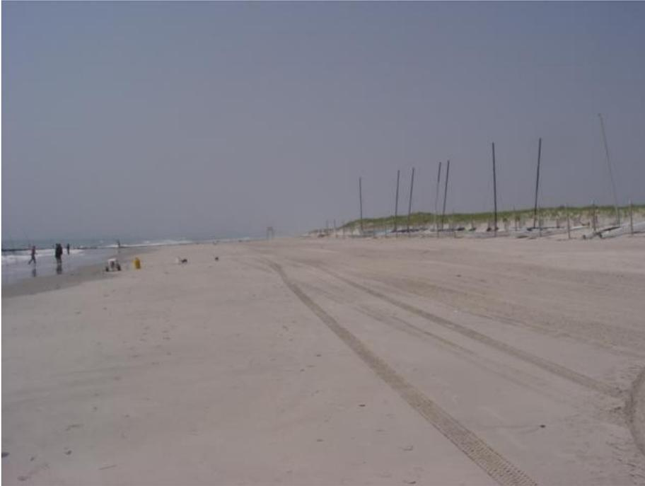
This beach is entirely composed of nourishment sand since the stone revetment was the principle barrier to wave damage prior to 1998. This June 8, 2007 picture shows that the rocks are buried and a dune grows over the revetment. The beach width has decreased slowly since 2003.
