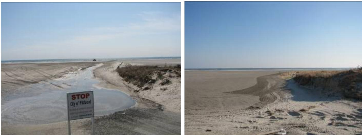
On April 4, 2012 the view across the beach in Wildwood was taken from the tiny dune in front of the boardwalk. The November 29<sup>th</sup> view on the right was taken from the same location, but minus the sign. The beach gained sand at the berm 600 feet seaward of the boardwalk. The sand deposit probably was derived from the erosion of the spring survey's berm.
