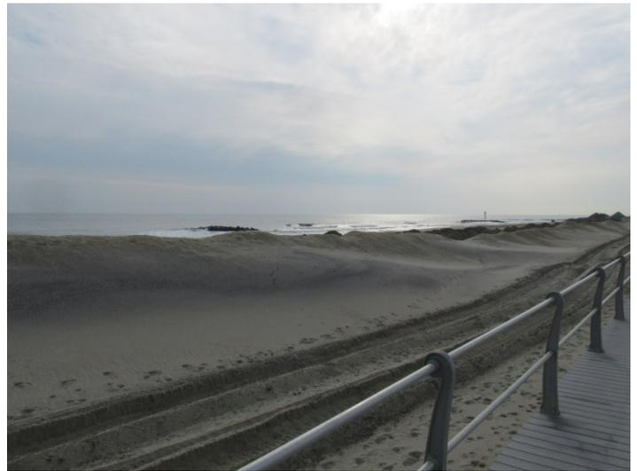
The USACE completed restoration in 2014 adding 32.29 yds<sup>3</sup>/ft. The view on December 11, 2015 shows a similar beach width with the winter storm “dune” in place seaward of the boardwalk. The vegetated dune still exists landward of the boardwalk.
