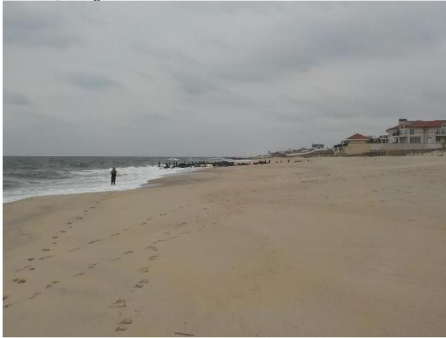
This site is located south of Lake Takanassee at a wide beach position south of the lake’s freshwater exit flume structure. The beach was 190 feet wide at elevation 10.0 to the berm crest. A year later the beach slope starts at the bulkhead and drops into the water with the 10-foot elevation berm gone.
