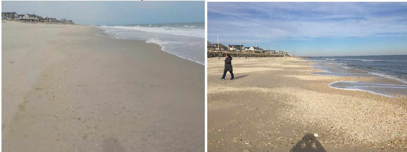
The Johnson Avenue profile contains no dune and a narrow beach (left photo taken January 19, 2018). The right photo (taken December 19, 2018) shows the exposed rock revetment. The position of the 0.0 ft NAVD shoreline moved landward (-33.0 ft) between surveys 55 and 57 and the berm lowered in elevation. Beach nourishment is scheduled for spring 2019.
