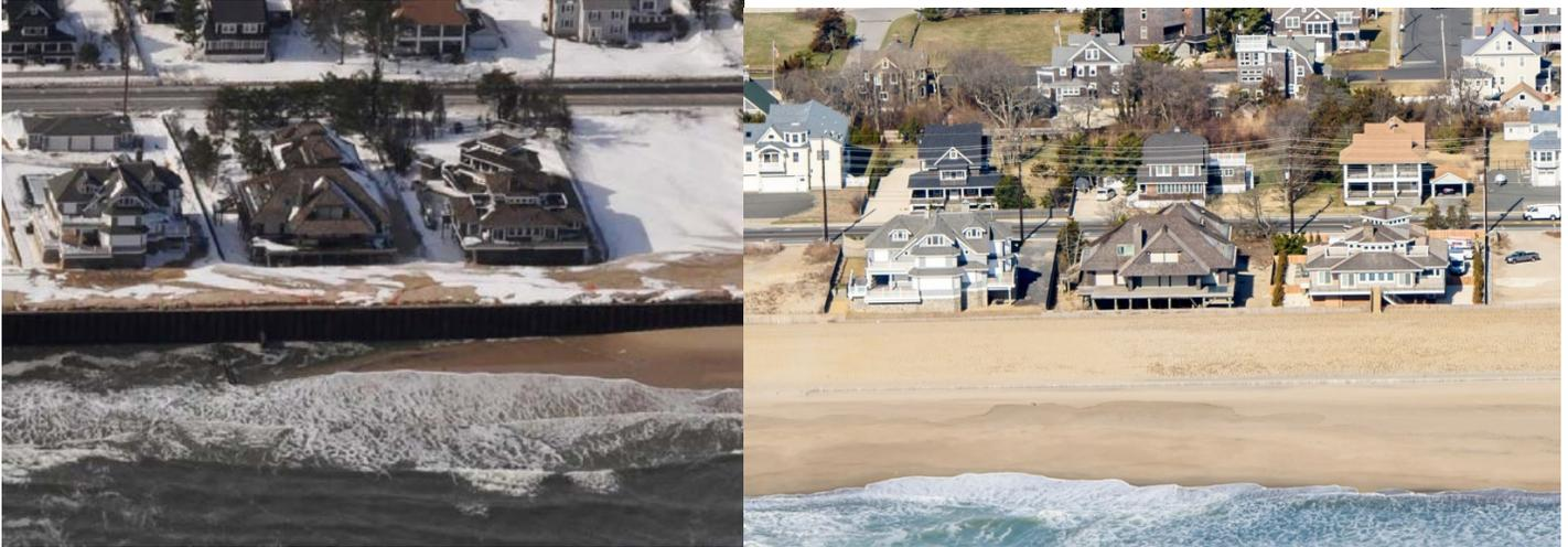
Figure 107. Direct comparison between a post-Jonas northeast storm on January 26, 2016, and post-beachfill project of the same three homes as of March 28, 2019 with the grass and fencing installed in Mantoloking near Herbert Street. The steel wall, installed in 2014 remains under the new dune crest as a final barrier to shoreline retreat.
