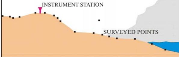
The profile survey continues until the swimmer reaches a depth of 15 feet, Mean Low Water. The survey is often carried out beyond -15 feet MLW. This happens when CRC personnel recognize the need to survey further to include a feature such as an offshore bar that may have migrated further seaward in response to a storm event.
