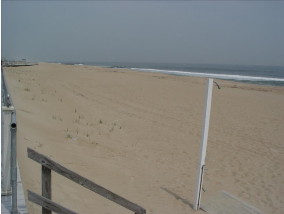
Figure 98. The May 5, 2006 photograph is of the beach between the boardwalk and the shoreline in southern Sea Girt. The slope up to the boardwalk has been filling in since the Federal project was completed. Keep in mind that in 1995 the high tide line was west of this boardwalk and it was about 10 feet down from its surface to the sand.
