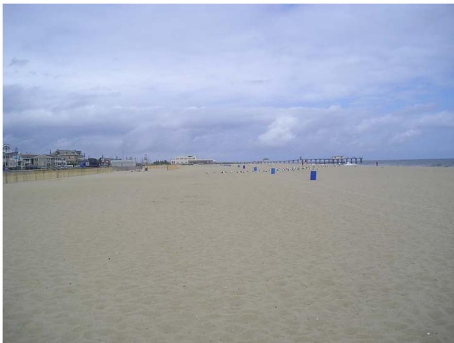
Figure 83. Located just south of Shark River Inlet, this beach has been at least 250 feet wide for decades due to the sand-trapping effect of the Shark River jetties. No nourishment sand was put here for that reason, but sand movement has added to the width over the past 7 years. The photograph was taken June 19, 2006.
