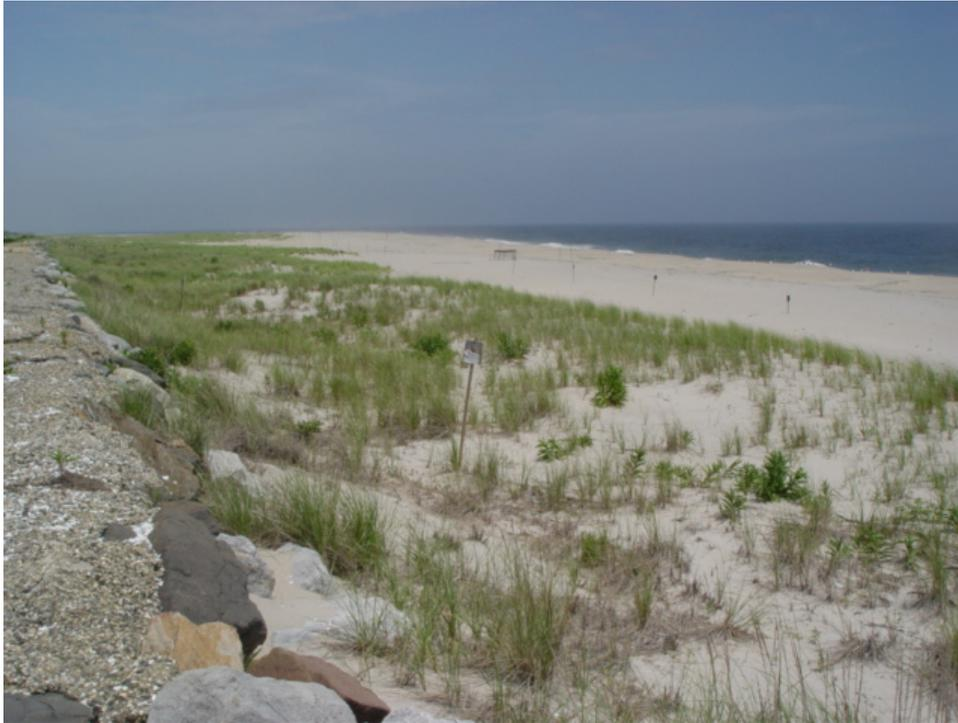
Figure 17. On June 27, 2006 the beach width was 150 feet. Substantial erosion took  $13.62 \text{ yds}^3/\text{ft.}$  from the berm and reduced its width by 100 feet. Some accumulation took place by the March 2007 survey.
