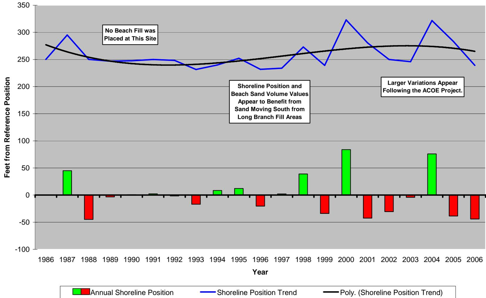
**Figure 41 – Site 171.** No sand was added to the Elberon beaches south of the West End Avenue site in Long Branch. The variability of the shoreline position grows dramatically larger in the years following the ACOE project to the north. The trend in position curves upward by about 20 feet in average shoreline position was influenced by two large sand volume input years (2000 and 2004).
