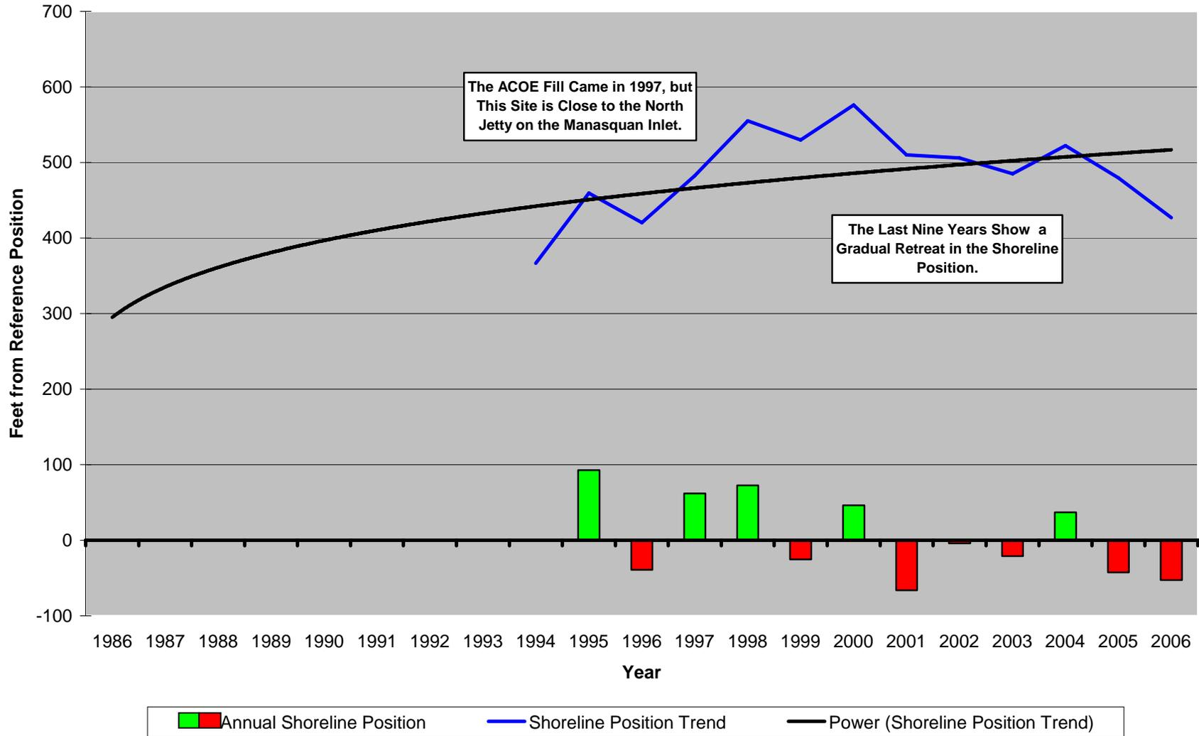
**Figure 71 – Site 256.** This profile was added in 1994 to provide closer coverage of the shoreline and sand volume changes on the north side of Manasquan Inlet. The sand volume added was reduced at the inlet because the jetties were shorter than necessary to retain the normal
