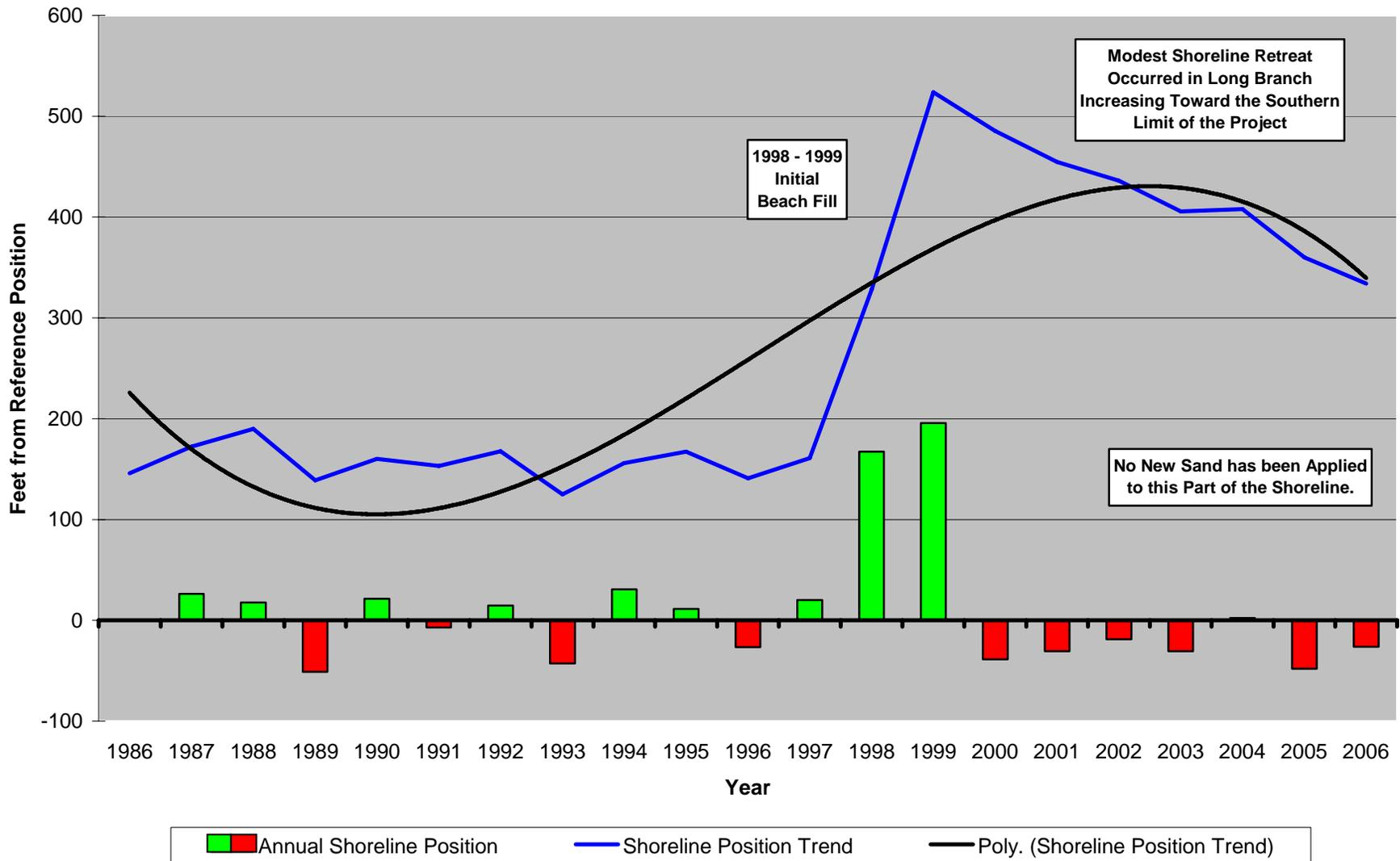
**Figure 37 – Site 174.** This profile in the middle of the Long Branch oceanfront begins to show an increased rate of shoreline retreat. The process is directly related to the fact that the initial project ended at the Long Branch southern boundary due to issues of real estate easements
