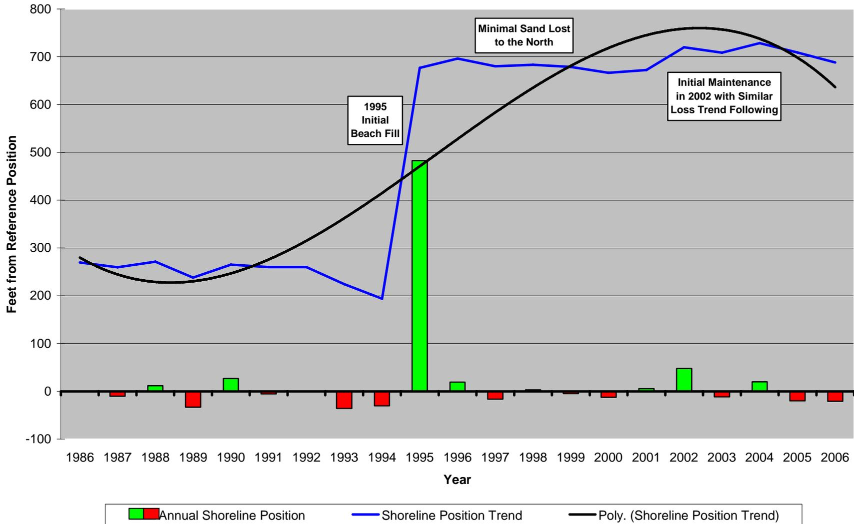
**Figure 21 – Site 182.** This profile is located between groins and as a result a beach did exist prior to the beach nourishment. The shoreline position shifted within a narrow range prior to 1995 and a trend of very minor shoreline retreat appears to be consistent following both the initial fill and the 2002 maintenance nourishment effort. The beach is heavily used recreationally during the season.
