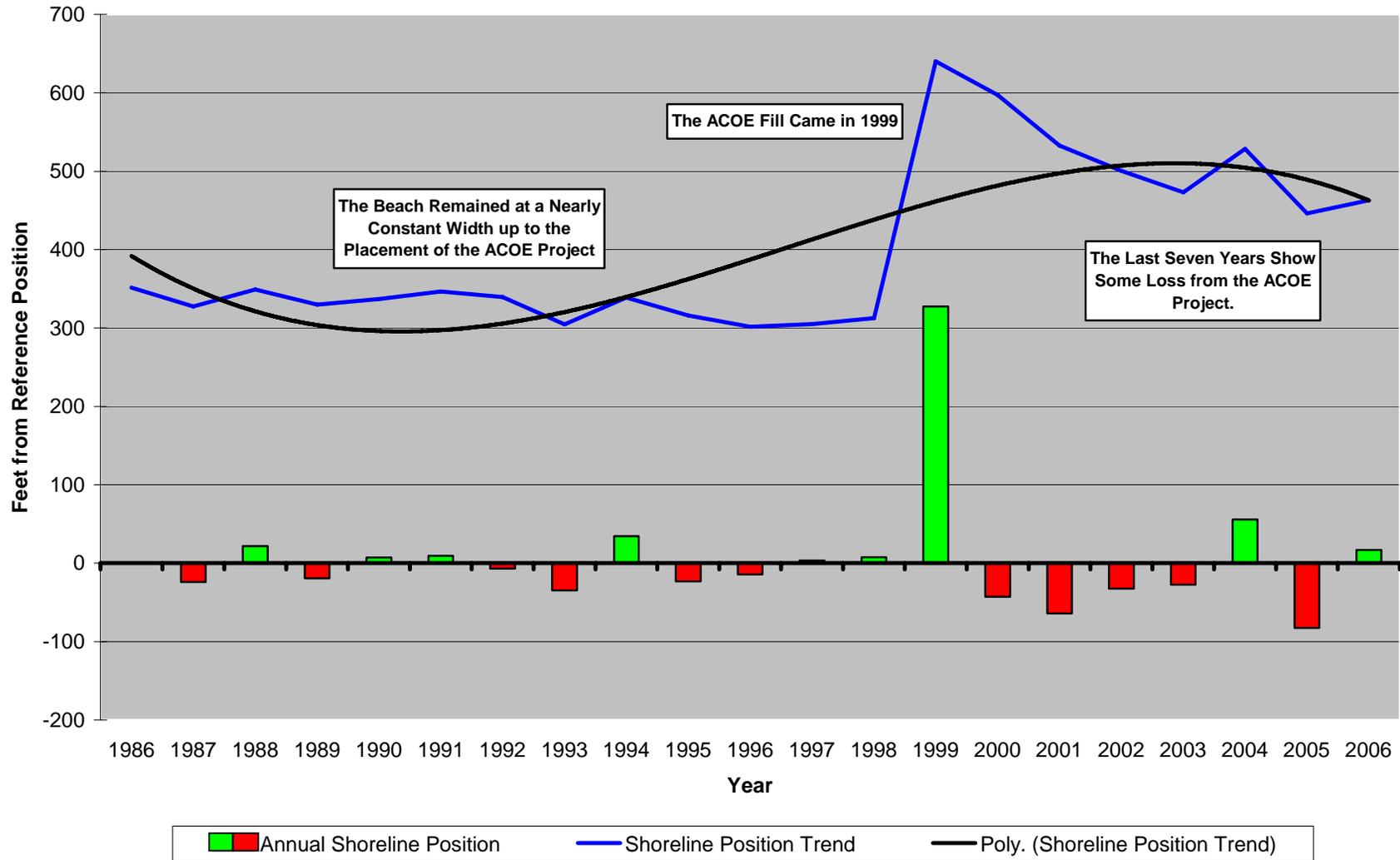
**Figure 53 – Site 166.** The extended period of slow shoreline retreat ended in 1999 with a better than 300-foot advance in the position with the fill project construction. Retreat occurred in 5 of the next 7 years to generate approximately 50% retreat in the 300-foot advance. The net change at this site since 1986 was an advance of 120 feet.
