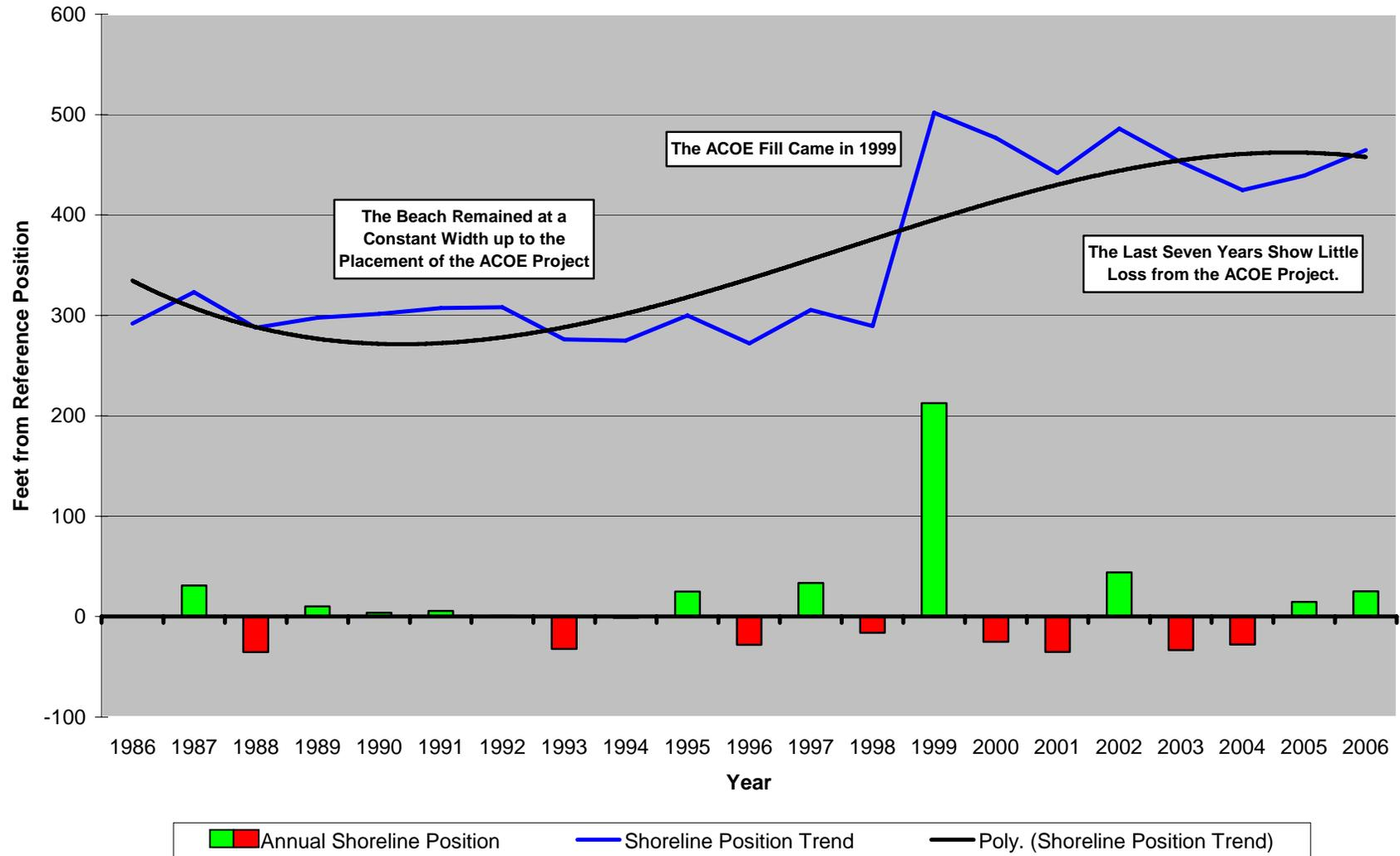
**Figure 51 – Site 167.** This profile is centrally located in Asbury Park, remained stable between 1986 and 1999. The 200-foot increase in shoreline width due to the fill has remained in place with only a 40-foot retreat in seven years. By 2006 the sand volume increase for the study period was 142.35 yds<sup>3</sup>/ft.
