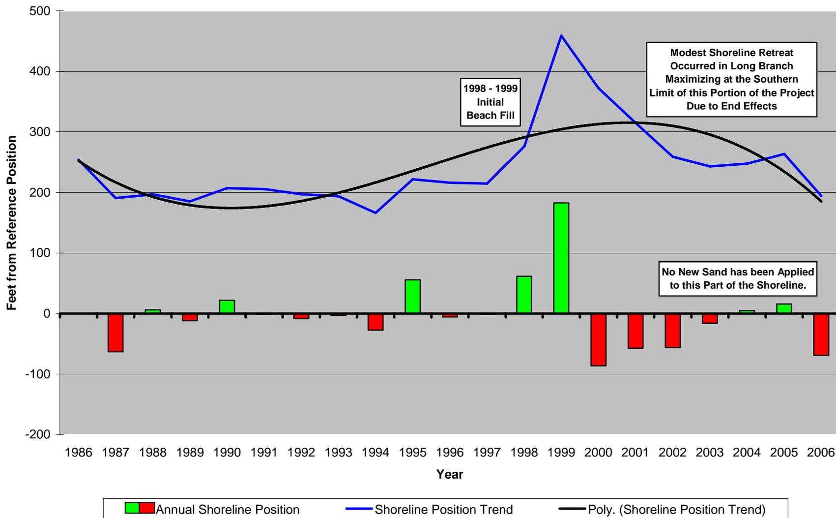
**Figure 39 – Site 173.** West End Avenue was essentially the southern limit of sand placement due to real estate issues blocking sand placement further south. The commencement of loss was immediate and continued at a constant pace until 2003 when a mild reversal
