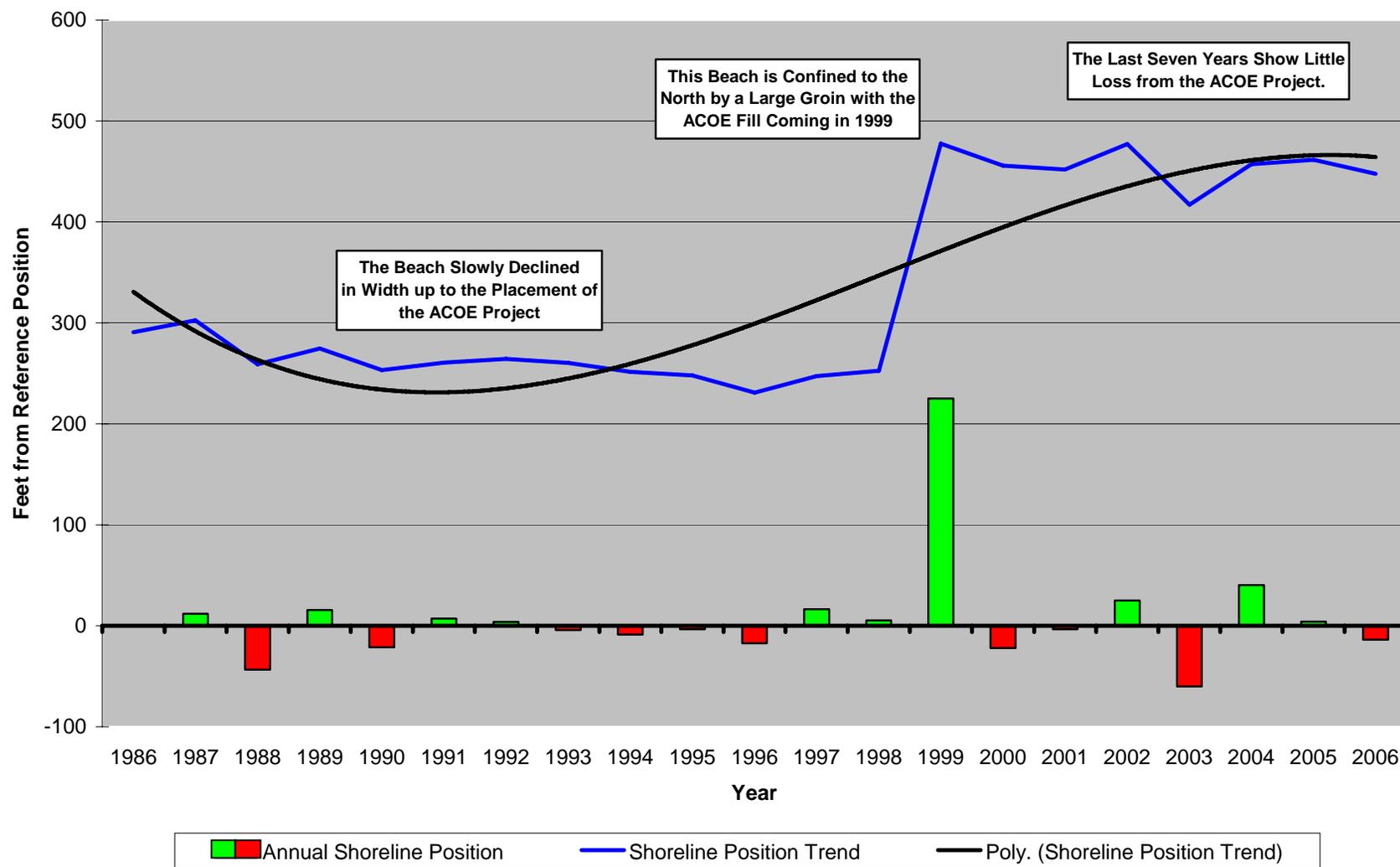
**Figure 49 – Site 267.** Located two blocks from Deal Lake in Asbury Park, the effects of the 1999 ACOE shore protection project are clear. In spite of the gains seen in Allenhurst offshore, the sand volume as shown by the shoreline position has remained fairly constant since 1999. No new sand has been added here since 1999.
