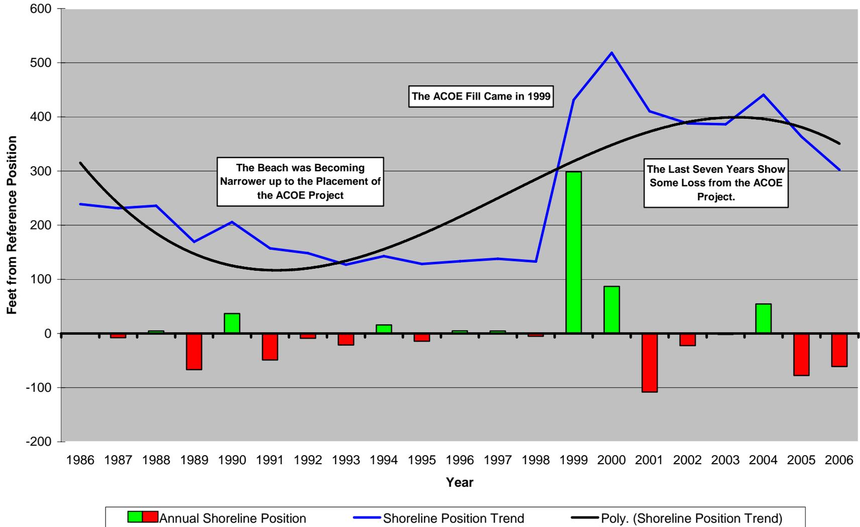
**Figure 55 – Sit e165.** The rate of shoreline retreat was greater in Bradley Beach than in Ocean Grove prior to the ACOE project. The 1992 storm forced the municipality to pull the boardwalk completely off the beach and move it onto the top edge of the bluff. This provided an
