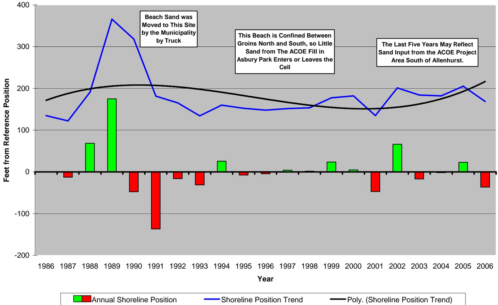
**Figure 47 – Site 168.** Positioned less than a mile north of Asbury Park where the ACOE project commenced south to the Manasquan Inlet, this Allenhurst site also shows a post-construction positive trend in shoreline position since 2000. The big spike in 1989 was due to the
