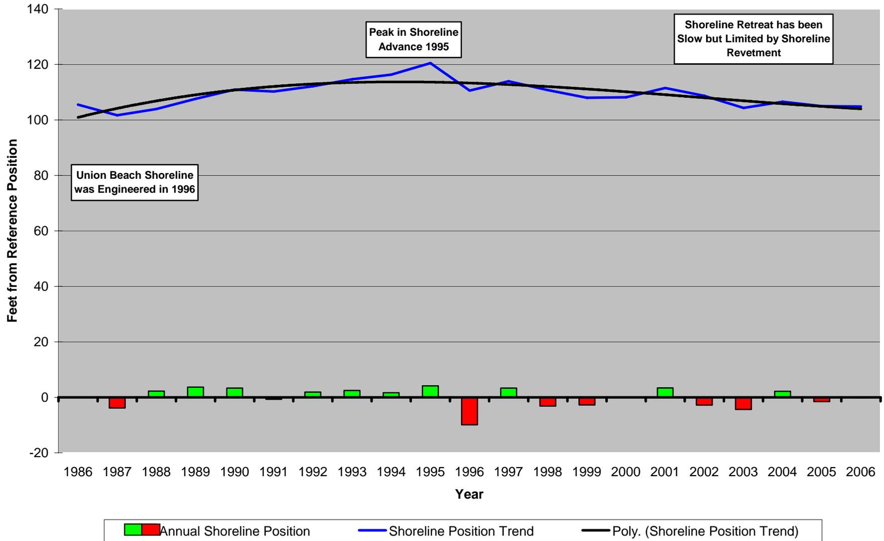
**Figure 7 – Site 186.** Union Beach is basically an engineered shoreline with a rock revetment constructed during the 1990’s and a small wet to dry beach at the base of the rocks. There is no dune and prior to the rock wall construction by the State, there were sections of the
