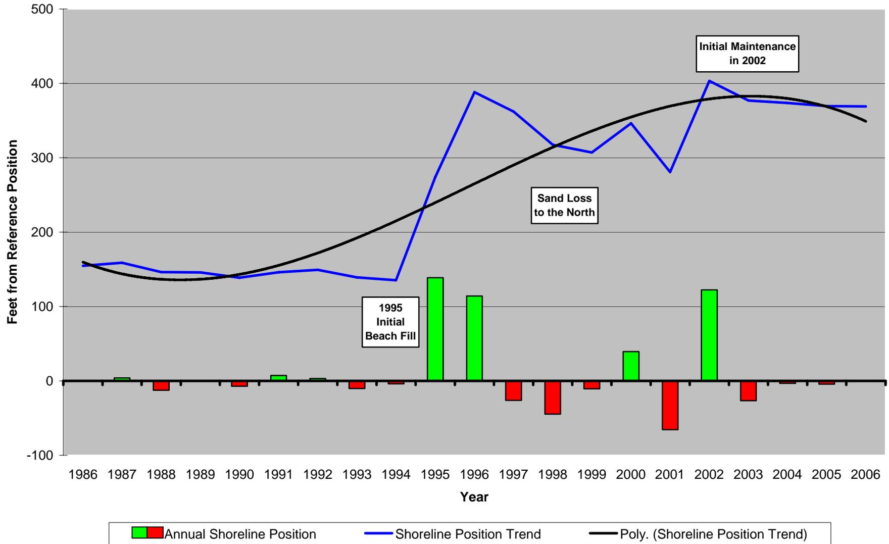
**Figure 15 – Site 184.** This profile was an example of how the Sea Bright seawall provided the only protection from storm damage along the northern 13 miles of Monmouth County prior to beach nourishment. There was no dry beach and surveys went from the rocks of the seawall
