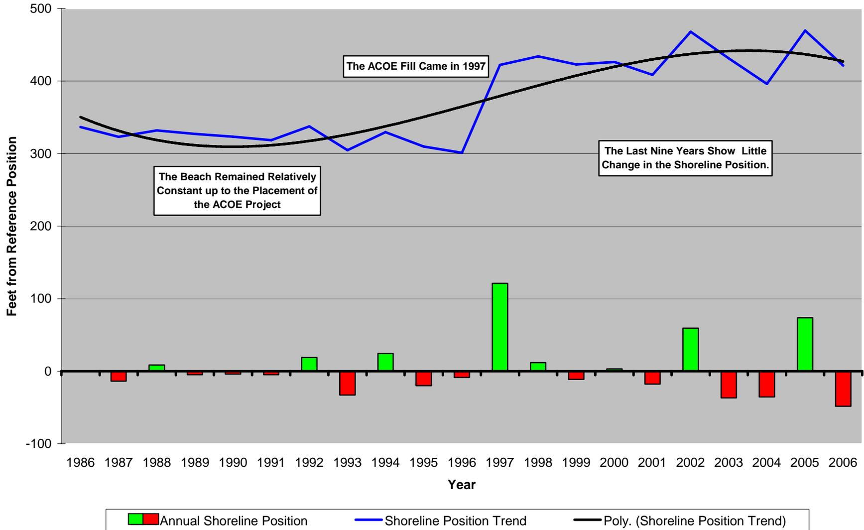
**Figure 65 – Site 160.** The Salem Avenue site demonstrated a very slow retreat in the shoreline between 1986 and 1996. The ACOE project produced a 120-foot advance that remained nearly constant until 2001 when a series of larger swings caused larger changes in the zero
