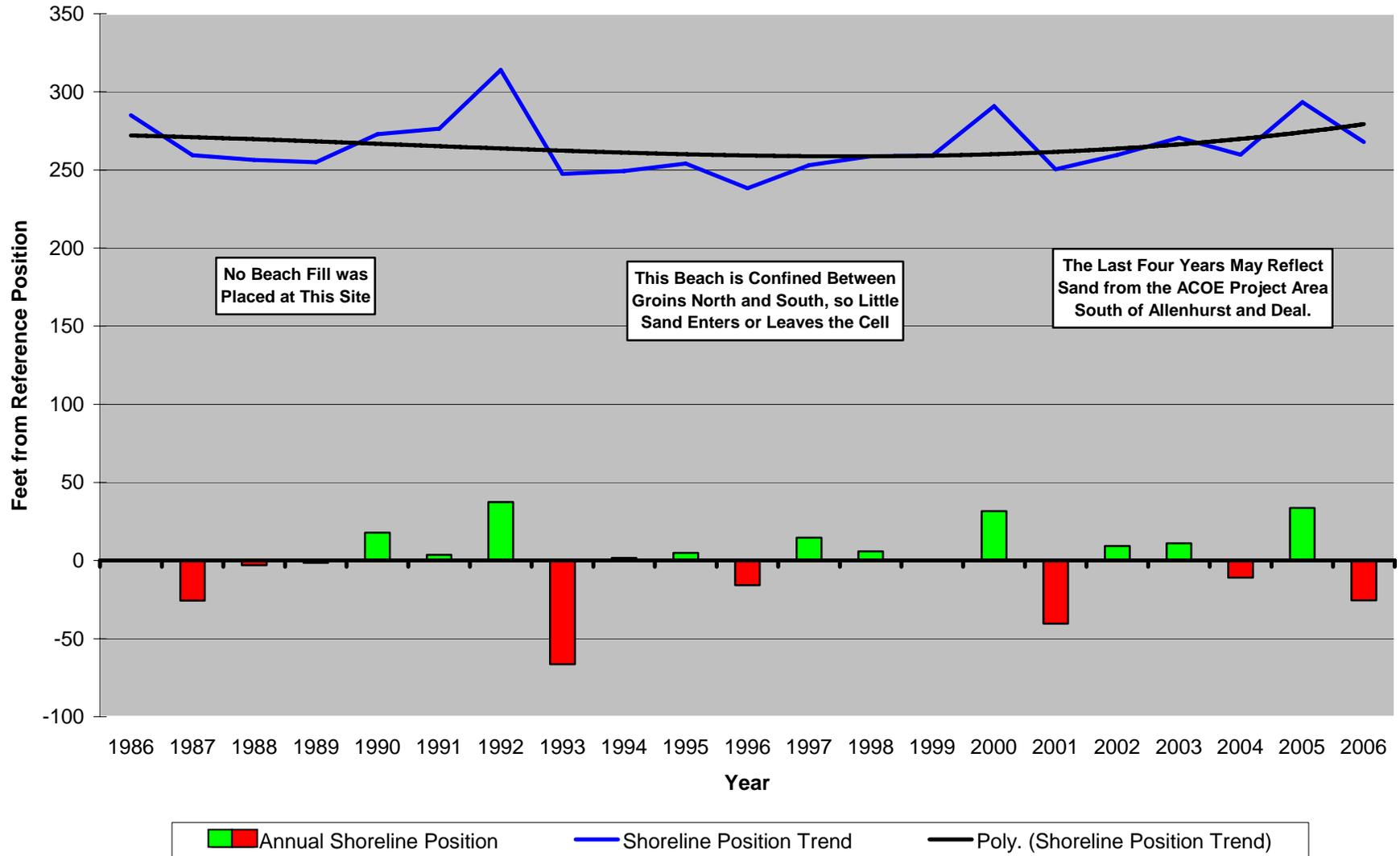
**Figure 45 – Site 169.** The Darlington Avenue site had more sand within the groin compartment than most other Deal shoreline segments. This is because the bluff was less protected from direct wave erosion, which over time introduces new sand to the system as the bluff
