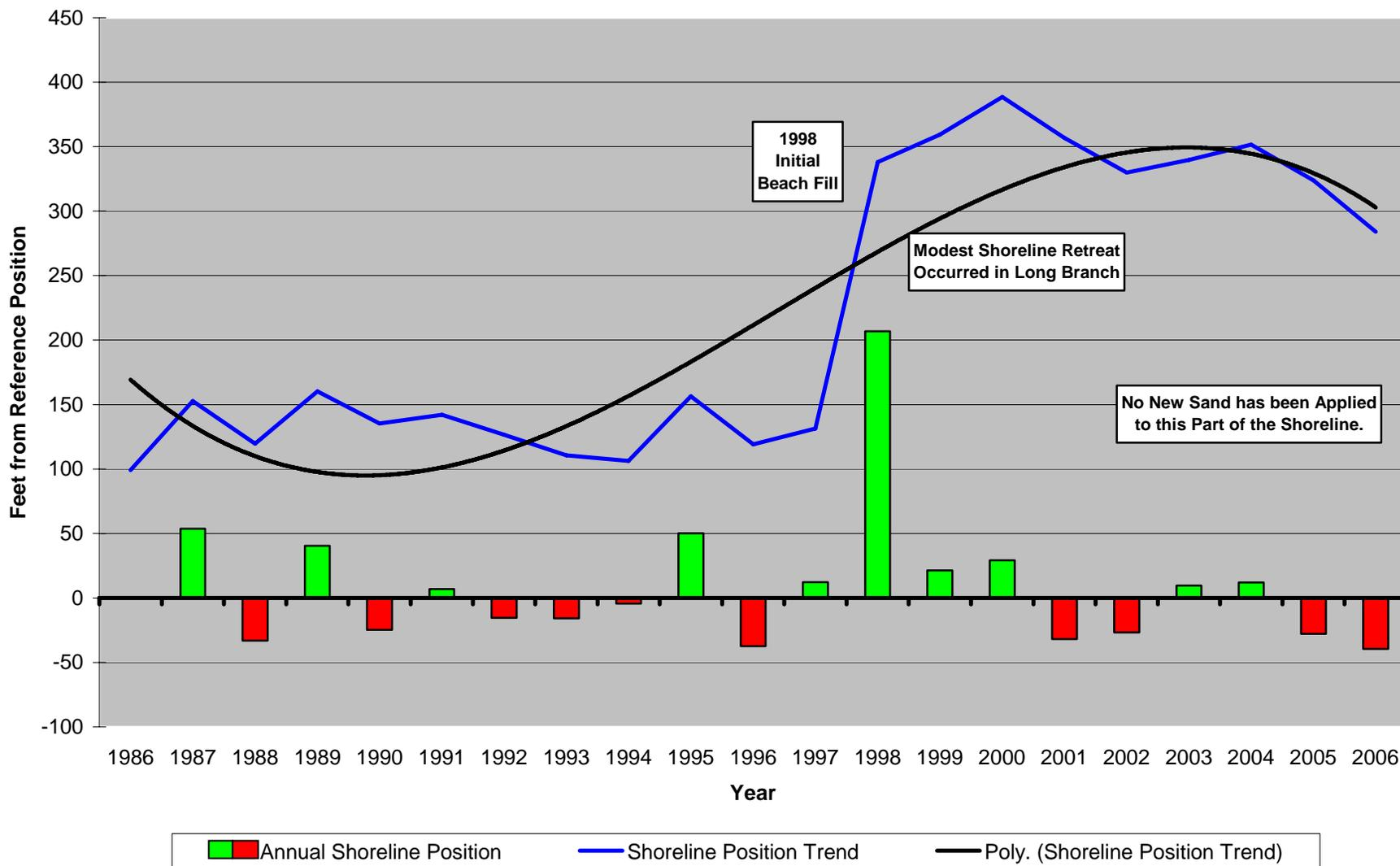
**Figure 35 – Site 175.** The major segment of the Long Branch shoreline is represented by cross sections #175 (this site), 174 and 173 where the uplands bluff was protected by a vertical steel bulkhead dating from the mid-twentieth century. Later the southern half was reinforced
