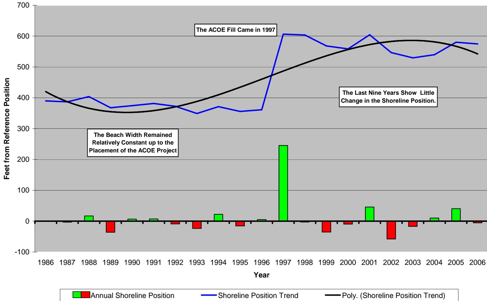
**Figure 65 – Site 159.** The 1997 fill produced over a 200-foot advance in the shoreline that has remained relatively stable for the last 9 years. The 2006 position is only 30 feet landward of the “as-built” location. The shoreline pattern fluctuated with 3 advances and 6 retreats post-construction, with relatively modest variations in width leaving the beach in excellent condition.
