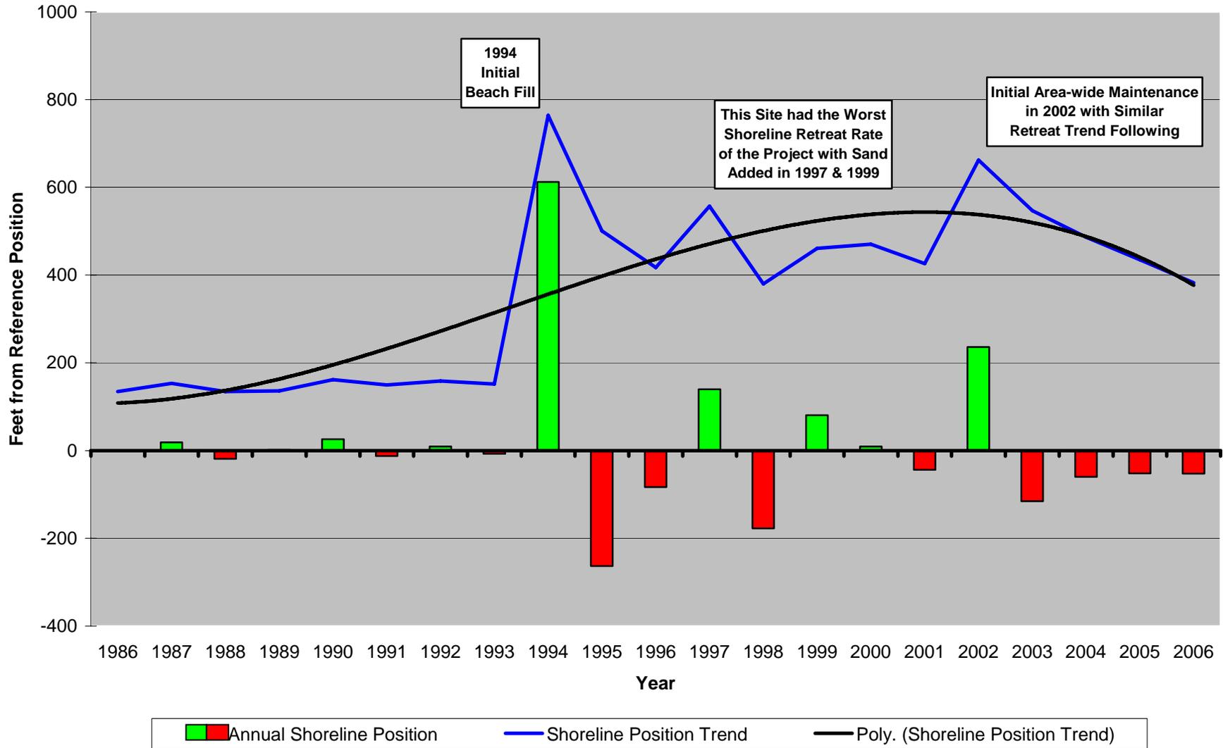
**Figure 27 – Site 179.** The Cottage Road site lies just north of a vintage beach club that was built seaward of the highway and protected by moving the seawall seaward around the structure. This geometry appears to enhance the erosion rate at this beach. The trend shows a substantially greater rate of retreat in the shoreline than at other Sea Bright sites. The dredge added sand in 1997 and 1999 as it was involved
