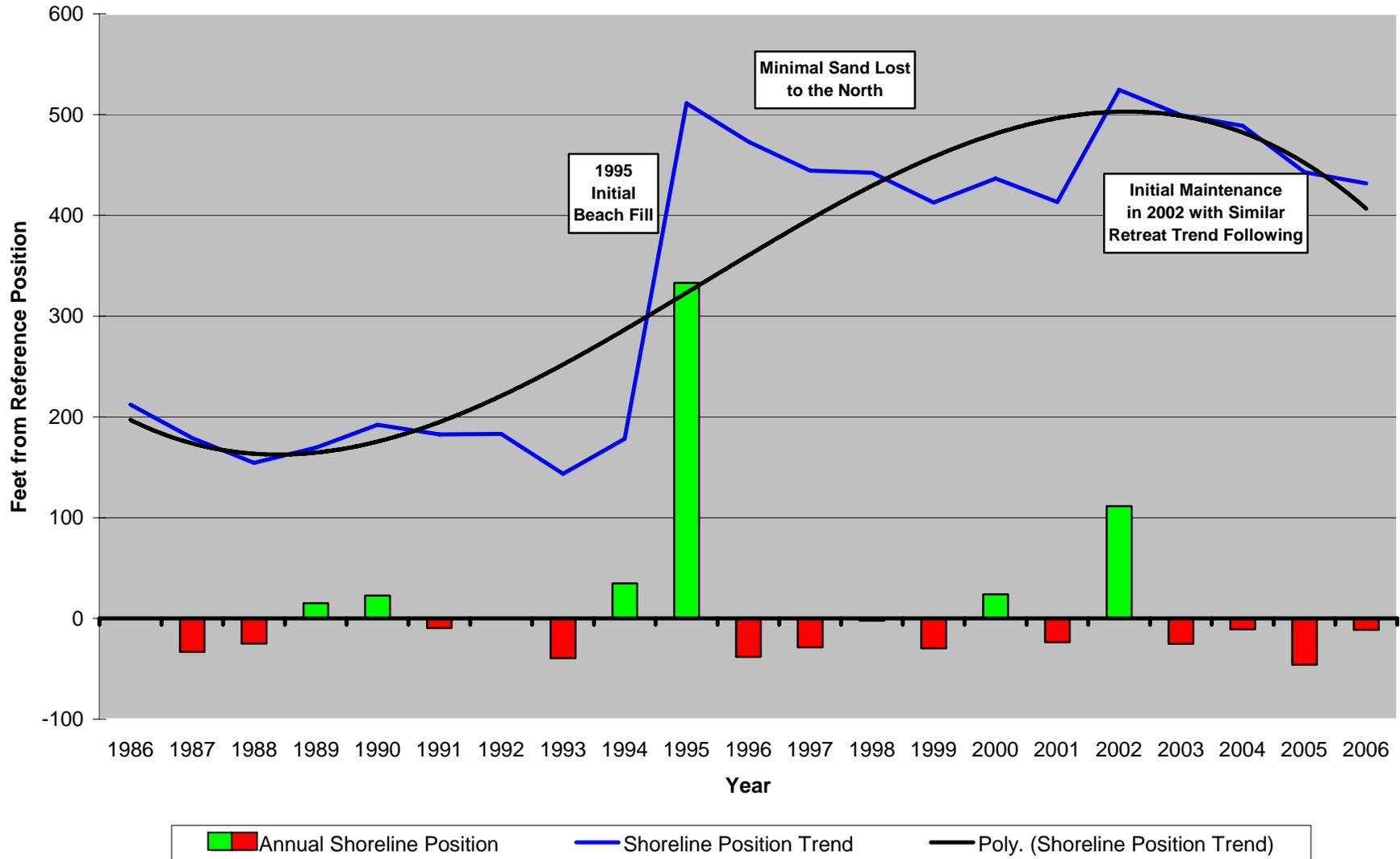
**Figure 25 – Site 180.** Further south along the Sea Bright shoreline the beach was very narrow in 1986 with sand banked up against the rocks and a beachface slope that began immediately seaward to the zero elevation line at a distance of 200 feet from the reference. Storms in 1991 and 1992 reduced this distance by 50 feet prior to the initial beach replenishment.
