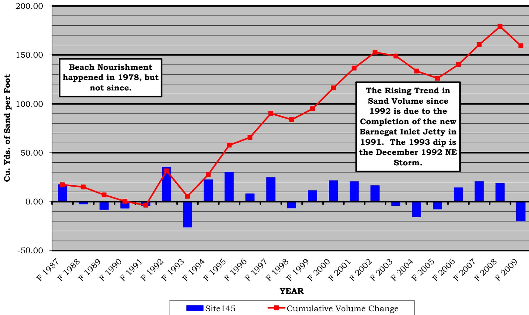
Figure 45. The new jetty at Barnegat Inlet produced a huge advance in the entire Borough shoreline since 1992. The amount declines slowly from 2,400 feet of advance at the jetty to about 60 feet at 26<sup>th</sup> Street. That advance added 160 cy/ft to the site's sand volume. The two locations either side of Barnegat Inlet had the highest values in shoreline advances in the county for 2009 (60 and 62 feet).
