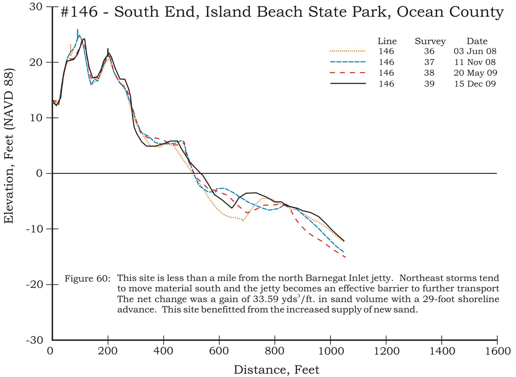
Figure 60: This site is less than a mile from the north Barnegat Inlet jetty. Northeast storms tend to move material south and the jetty becomes an effective barrier to further transport. The net change was a gain of 33.59 yds<sup>3</sup>/ft. in sand volume with a 29-foot shoreline advance. This site benefitted from the increased supply of new sand.
