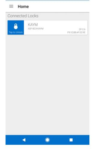
4. Once it is on your screen, while holding the lock in your one hand, click the blue tap to unlock icon, and wait until the indicator turns green. Immediately pull open the lock.
